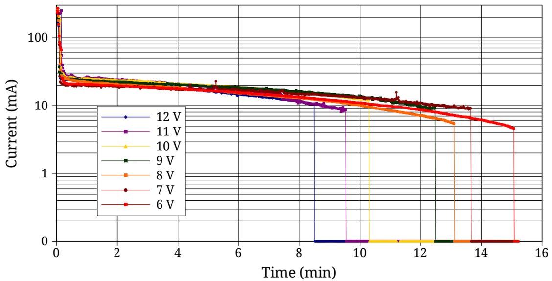
Figure 4.6: Etching with different potentials
