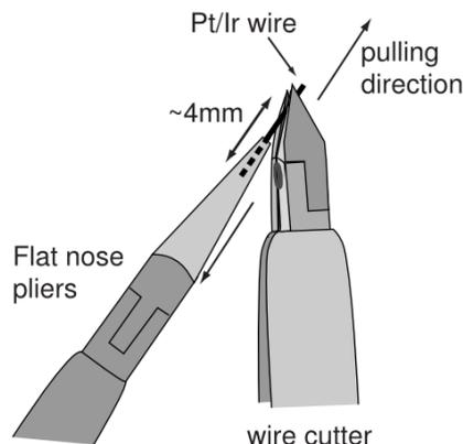
Figure 3.2: Schematic view of Pt/Ir wire cutting [23]
