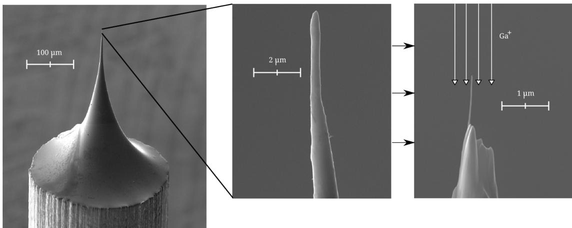
Figure 4.13: Etched tungsten tip sharpened by FIB.
