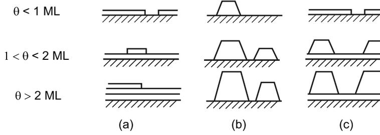
Figure 2.3: Schematical presentation of three growth models as a function of  $\Phi$  monolayer coverage (ML) (a) layer on layer (b) islandes (c) layer and islands[19]
