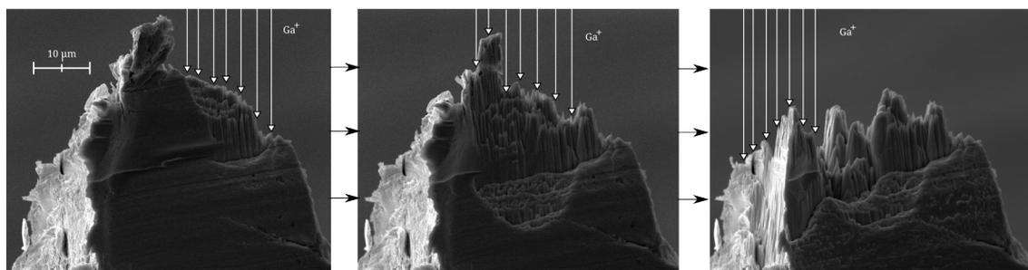
Figure 4.15: Three pictures show SEM view after three steps of  $\text{Ga}^+$  beam scattering of Pt/Ir. For original view refer to figure 4.11
