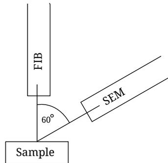
Figure 4.12: Schematic view of Tescan<sup>®</sup>SEM-FIB combined microscope LYRA 3 FIB-FESEM
