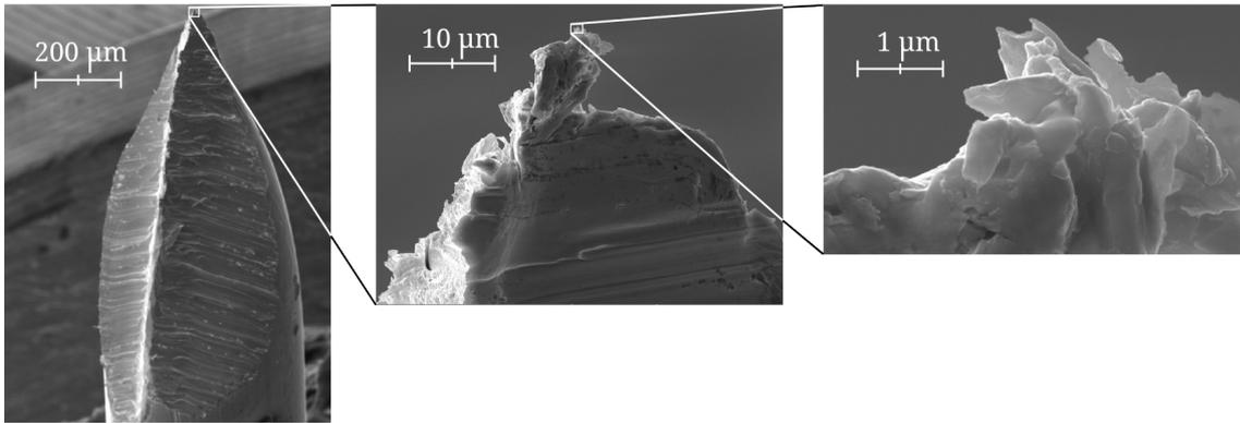
Figure 4.11: SEM analysis of a Pt/Ir cut tip
