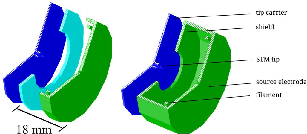
Figure 4.16: Analysed geometries of the system for tungsten tip decontamination. Simulations in EOD<sup>®</sup>. Left is the setup with separated shield and source, right is the compact setup.
