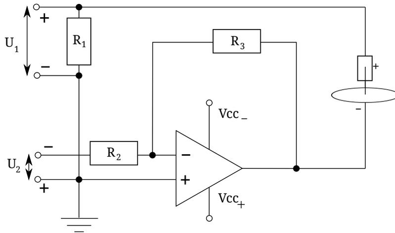
Figure 4.2: Schematic view of the circuit employed in figure 4.1 in order to magnify the potential output of the PC card.  $U_1$  represents the potential measured in order to acquire current flow.  $U_2$  is the potential output from the PC card.  $V_{cc\pm}$  is the amplifying potential of 15 V. The resistors are  $R_1 = 250 \Omega$ ,  $R_2 = 1 \text{ k}\Omega$ ,  $R_3 = 500 \Omega$ .
