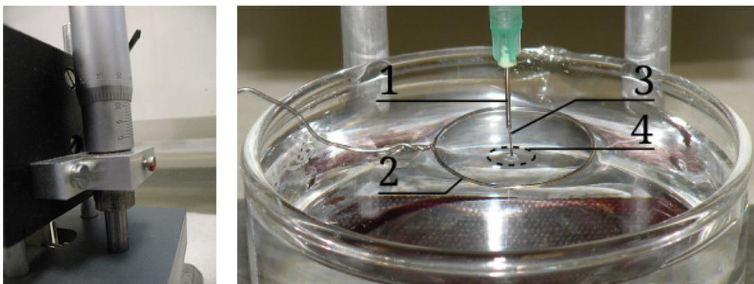
Figure 4.4: Details of the apparatus. On left side is the micrometer gauge. On the right side is a detail from the static electrochemical etching setup in figure 4.3. (1) hypodermic needle serving as a support for the tungsten wire, (2) stainless steel ring, (3) tungsten wire, (4) meniscus.
