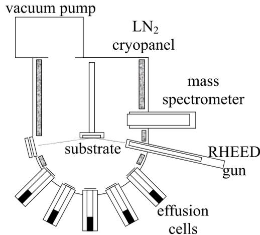
Figure 2.2: Cell for Molecular Beam Epitaxy[27]
