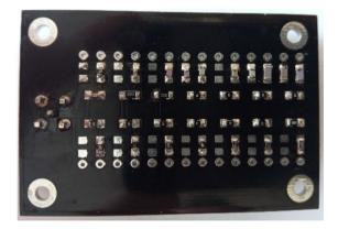
**Fig. 8** Photograph of one side of two-sided PCB developed to carry up to 86 (14 branches each consist of 6 passive slots plus 2 slots for correction elements) passive components approximating our CPE (CPE30)
