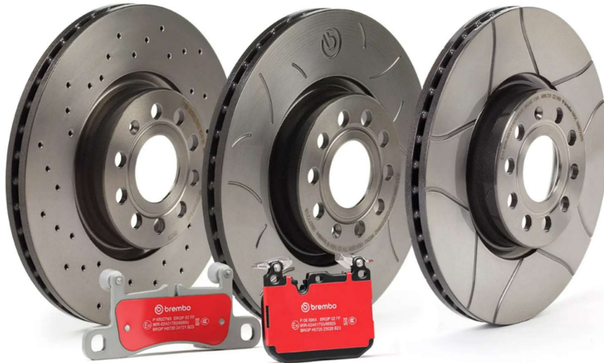
Figure 2.3: Drilled brake disc on the left, variations of the slotted brake discs in the middle and on the right [7]
