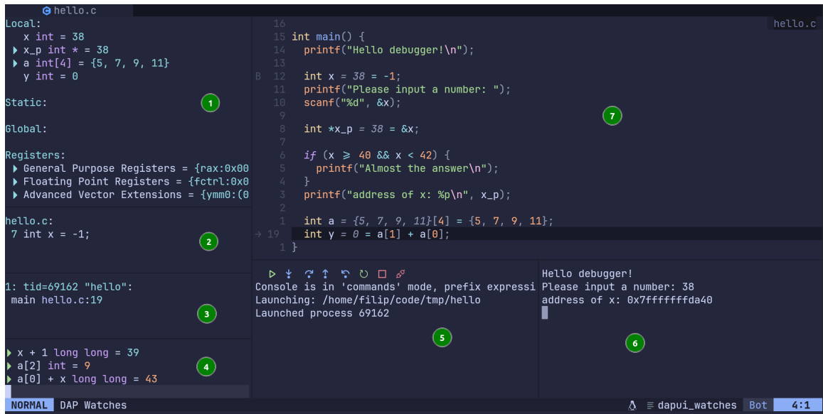
Figure 4.1: Screenshot of an integrated source-level debugger. The debugger presents a user interface inside the development environment. It is split into multiple parts: (1) view of variables and their scope, together with the current state of registers, (2) list of set breakpoints, (3) function call stack, (4) the watches window, (5) buttons for execution control and a debugger console, for issuing commands, which are not made available through the UI, (6) output and input of the program, (7) view of the source code, annotated with breakpoint positions, variable values and an indicator of which line will be executed next (line 19).
