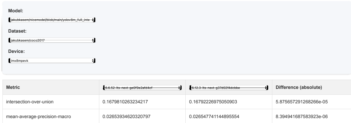
Figure 7.3: The accuracy comparison interface displaying results for the YOLOv8 model and the Coco2017 dataset.
