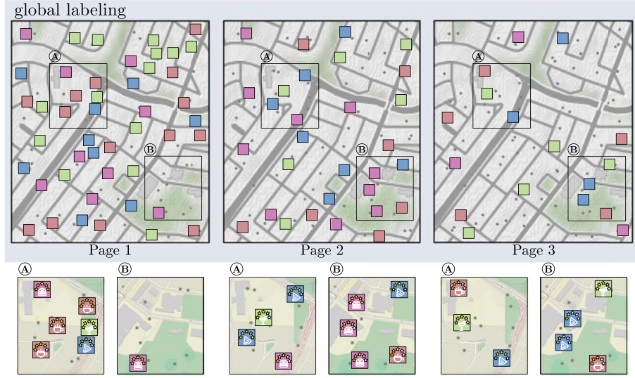
Figure 2.7: An example of a small-screen device approach consisting of three global labeling pages with an illustration of two local labelings (A, B) proposed by Gedicke et al. [59]. Time-consuming global labelings are pre-computed during a preprocessing phase, done once, and then local labelings are extracted during a query phase. In the query phase, local labeling is achieved by sampling all labels contained in the frame representing the current region of interest for each page.
