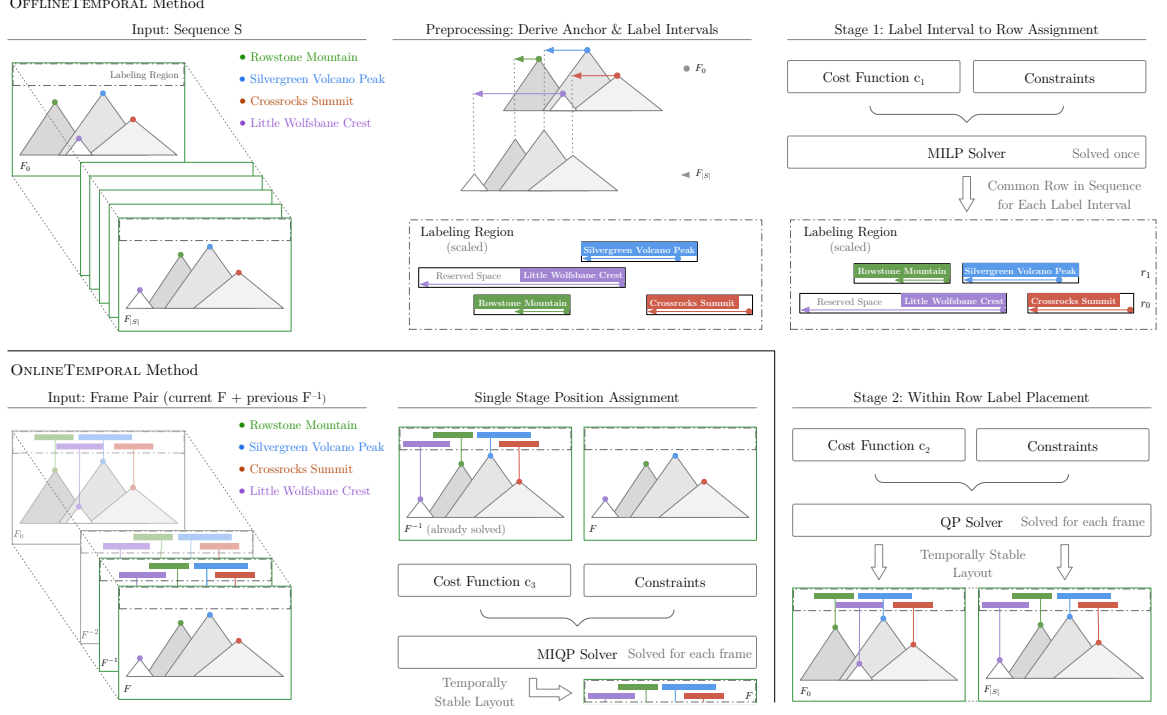
Figure 3.2: High-level overview of processing stages applied in the proposed methods. The OFFLINETEMPORAL method consists of the preprocessing stage followed by the Label Interval to Row Assignment and Within Row Label Placement stage. The ONLINETEMPORAL is designed as a single-stage method.
