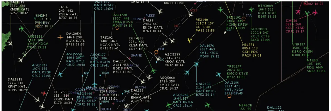
(b) Air traffic control (ATC) radar and onboard radar beacon transponders work together to display aircraft information on a radar screen. Each aircraft is represented by a symbol indicating direction and status. Information shown includes call sign, altitude, speed, origin, destination, and type. Symbols indicate if the aircraft is climbing or descending. Different colors represent arrivals, departures, and traffic to nearby airports [164].
