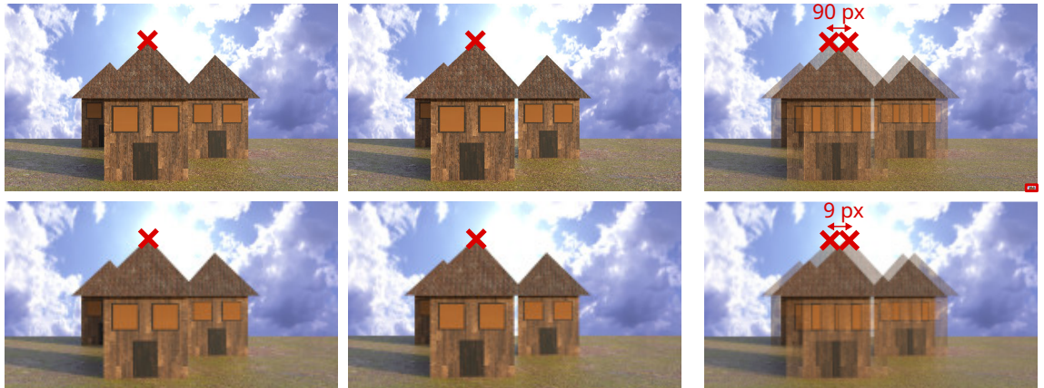
Figure 2.31: Search windows used to find the corresponding features in two views might not be optimal for high-resolution inputs. The image can be downsampled to reduce the distance in pixels between the features. Important details might be lost in such process due to the general loss of information introduced by downsampling. The figure shows the original and 10\times downsampled views. Right bottom corner of the original blended image (top-right image) shows the size of their difference.
