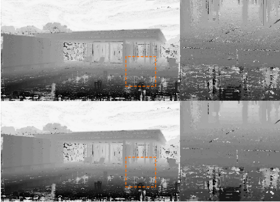
Figure 3.5: The noise in focus map resembles salt-and-pepper noise. Median filtering can be used to get rid of incorrectly focused pixels.
