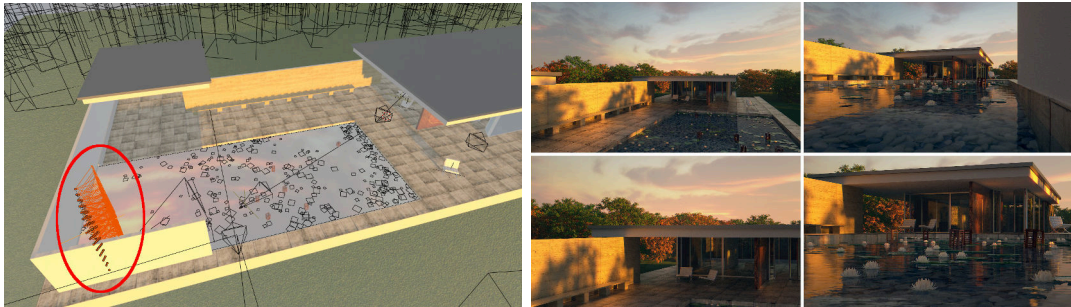
Figure 3.24: The size of the grid (red circle) in Pavilion scene and the value of field of view was animated and resulting reconstruction quality was measured. Two views from the corners of the grid using 25 mm focal length are placed in the middle and 55 mm ones at the bottom. The difference between views is bigger in the 55 mm version.
