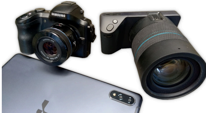
Figure 2.35: Three devices able to capture light field data are displayed in the photo. It is a standard Samsung Galaxy NX camera with 3D stereo lens, Lytro plenoptic camera, and 3D stereo camera on Leia LumePad 3D tablet.
