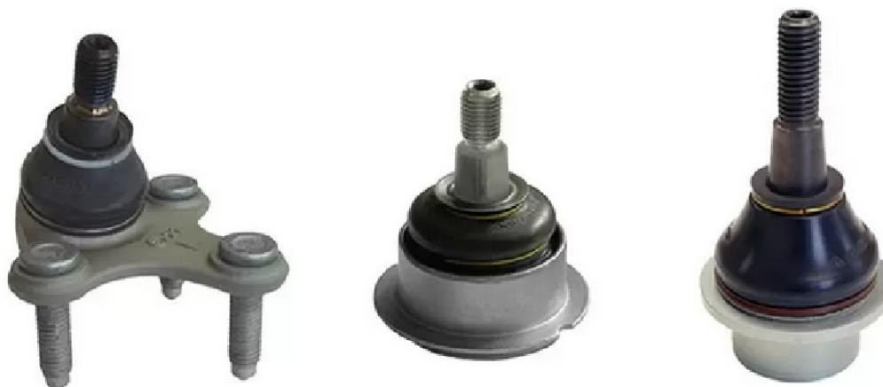
Figure 1.10. Wheel suspension ball joints. [8]
