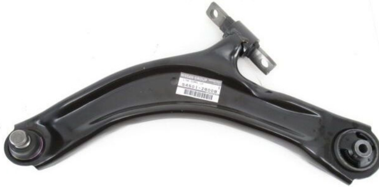
Figure 1.8. Lower control arm of vehicles suspension system. [6]
