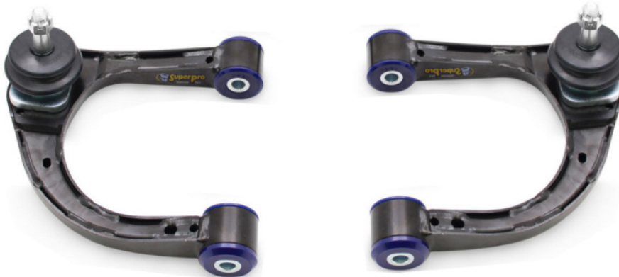
Figure 1.9. Upper control arm of vehicles suspension system. [7]
