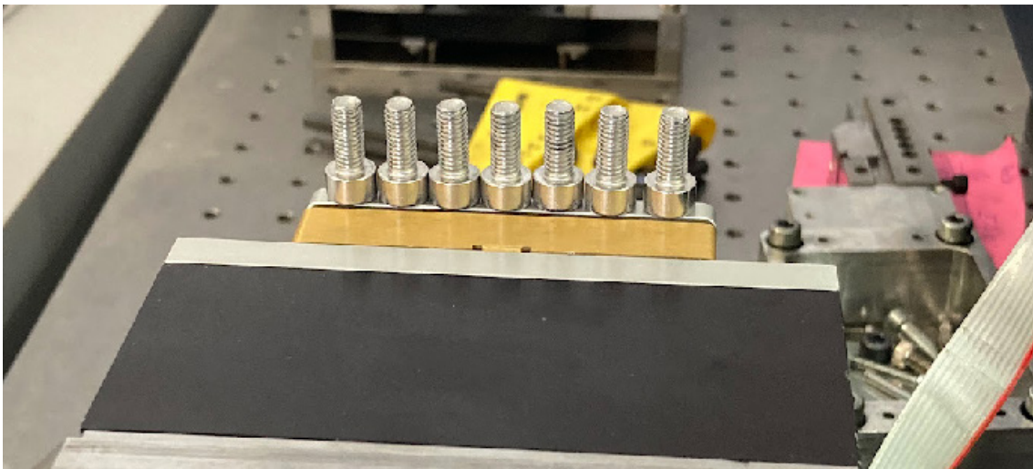
Figure 4.10. Screws placed on the sensor, which is positioned on its side.
