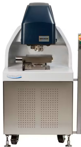
Figure 4.6. Optic profilometer Bruker Contour GT-X8. [58]
