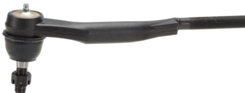
Figure 1.12. Outer tie rod of vehicle's steering system. [9]
