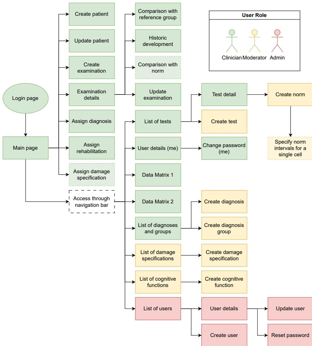
Figure 5.4: All the views implemented in the system and the manner in which users are expected to navigate through them. The elements with dashed borders represent views that are implemented in the form of a dialog.
