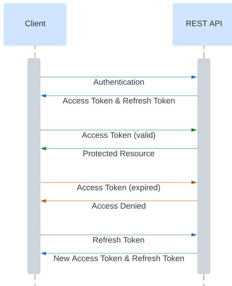
Figure 6.3: A sequence diagram of the JWT authentication and authorization process. The diagram uses a color scheme to differentiate between the types of requests. Blue represents authentication, green indicates successful authorization, and red unsuccessful authorization.<sup>18</sup>
