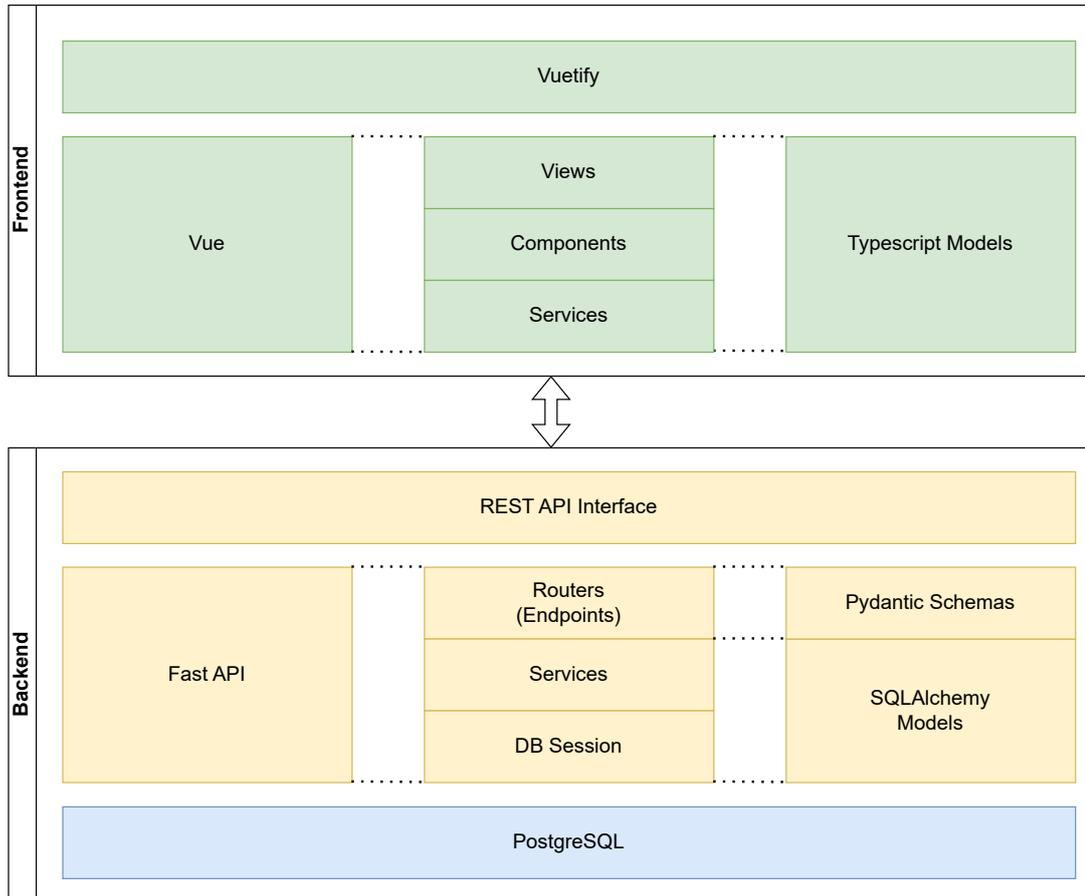
Figure 6.1: The architecture of the implemented system. The frontend communicates with the backend through a REST API interface.
