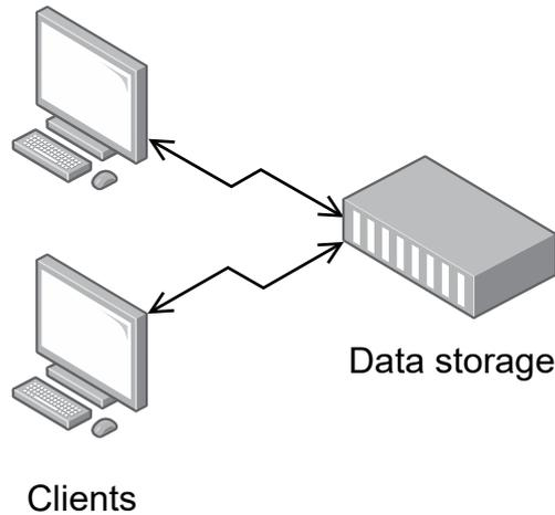
Figure 3.2: In the two-tier architecture, clients have direct access to the centralized data storage [27]. The data storage server is the only component responsible for handling client requests.
