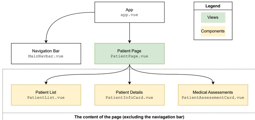
Figure 6.2: The hierarchical structure of Vue components on the main page (see Figure A.1) of the application. The `PatientPage.vue` file is located in the `views/` folder, while the remaining components highlighted in yellow are located in the folder `components/`. Note: Although all elements in this diagram are technically Vue components, the diagram distinguishes between *views* and *components* in the way they are used within the context of the application.
