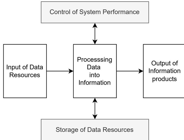
Figure 3.1: A diagram of control activities that process and transform data resources into information products [24].
