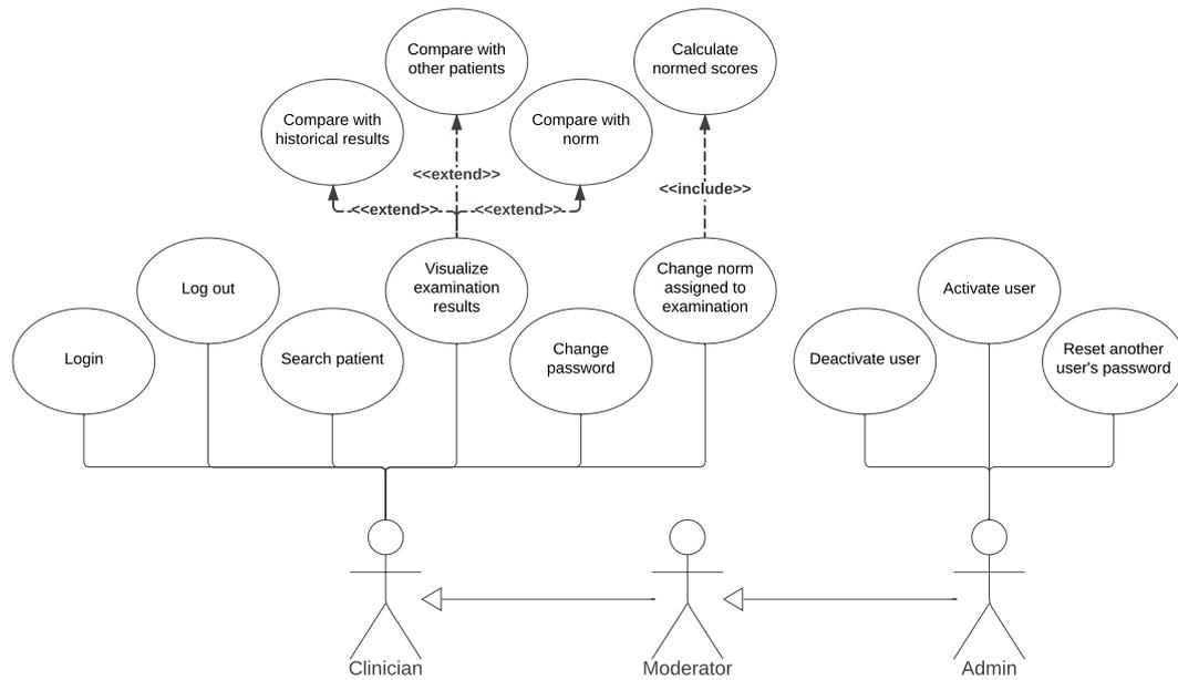
Figure 5.2: The use case diagram of the system. The use cases are not exhaustive, as operations that directly manipulate database entities were omitted for the sake of simplicity. These operations are presented in Table 5.1.
