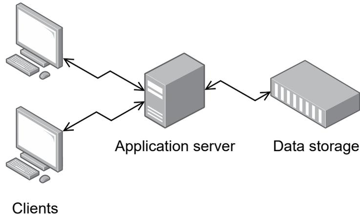
Figure 3.3: In the three-tier architecture, the application server acts as a connector between the clients and the data storage server, isolating them from each other. The figure is an adaptation derived from [27].
