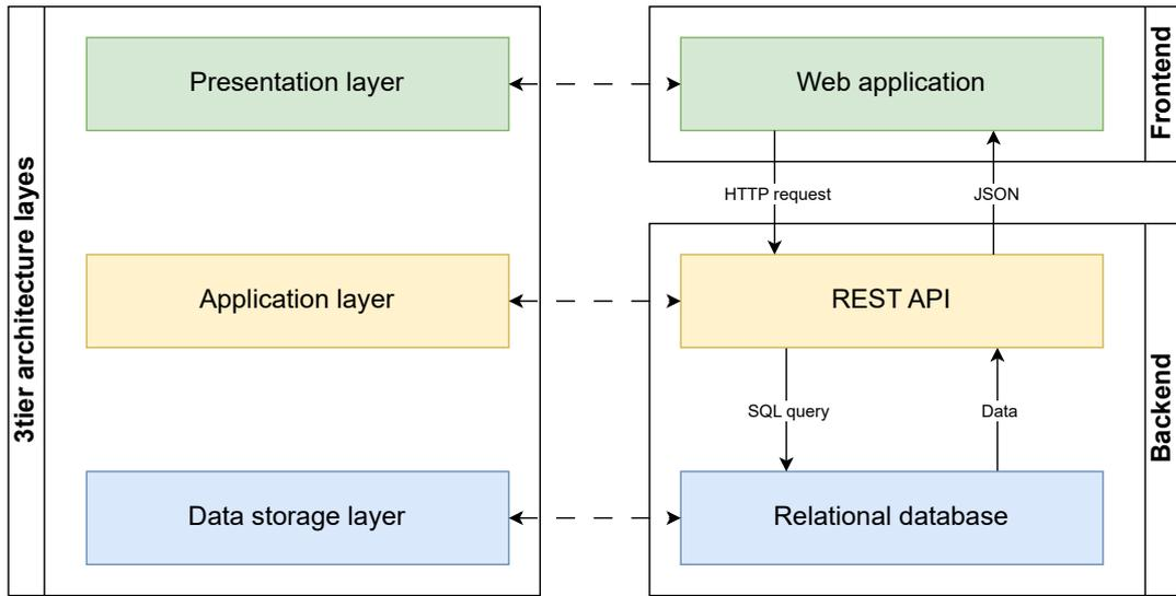
Figure 5.1: The architecture of the proposed system is based on an adaptation of the three-tier architecture. The REST API serves as an interface for clients to manage data in the database.
