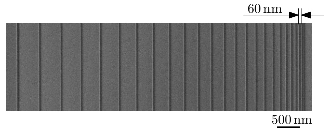
Figure 4.5: The resolution test prepared by focused electron beam-induced deposition using PMCPS precursor to test the lowest periodicity of the sinusoidal modulation that can be prepared using this technique. The pattern consists of 25 lines with different distances. The distance between the two lines is changing from 500\text{ nm} to 40\text{ nm} by 20\text{ nm} . The number of scans per line was N = 2\,000 scans. The energy of electrons was 30\text{ keV} , and the beam current measured in the Faraday cup was 542\text{ pA} .
