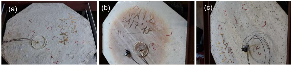
Fig. 18: Photo documentation of tested slabs. (a) 1AeA-N crack formed over the whole slab during the cooling period; (b) 2AeA-MC heated surface where the polymer microspheres coloured the non-heated surface; (c) 3AeA-Si cracked formed on the non-heated surface during the cooling period.
