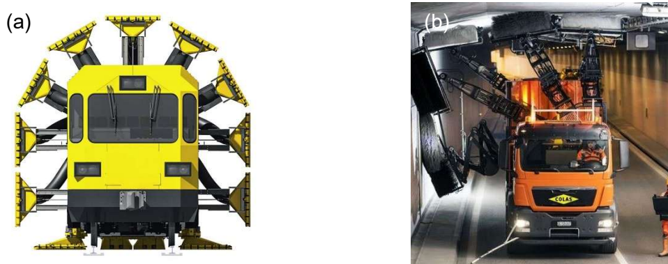
Fig. 16: Example of truck for application of IHT method: (a) for train tunnels; (b) for road tunnels.
