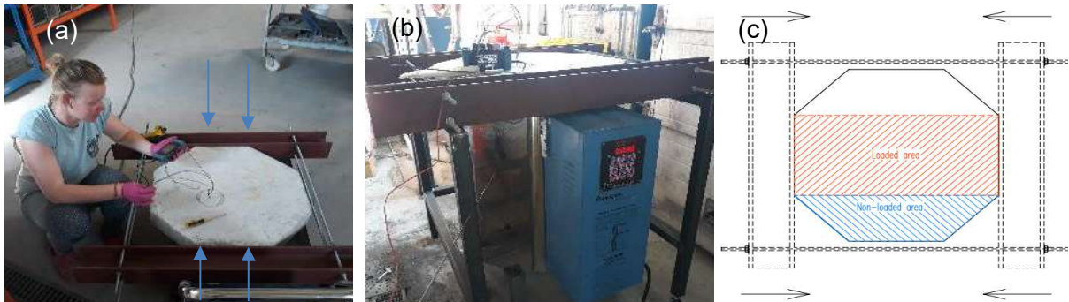
Fig. 4: Test setup for large scale one-side heated uniaxially loaded slabs: a) Uniaxial loading steel profile HEB 100 with prestressed treaded rods, assembling thermocouples and plugging in thermometer log; b) Testing slab placed on load-bearing frame and connected to thermal log; (c) Schematic drawing of the test slab: The uni-axial loading is applied in central area due to the shape of tested slabs.
