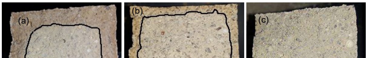
Fig. 10: Photo documentation of samples after thermal exposure according to m-ISO: (a) Ref sample; (b) IHT200/1; (c) IHT200/2.
