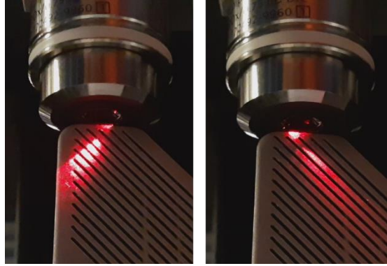
Figure 3.5 Measurement of maximal incident angle. The grid under the objective has 45° stripes. The laser beam can be tilted by objective up to 48.6°.
