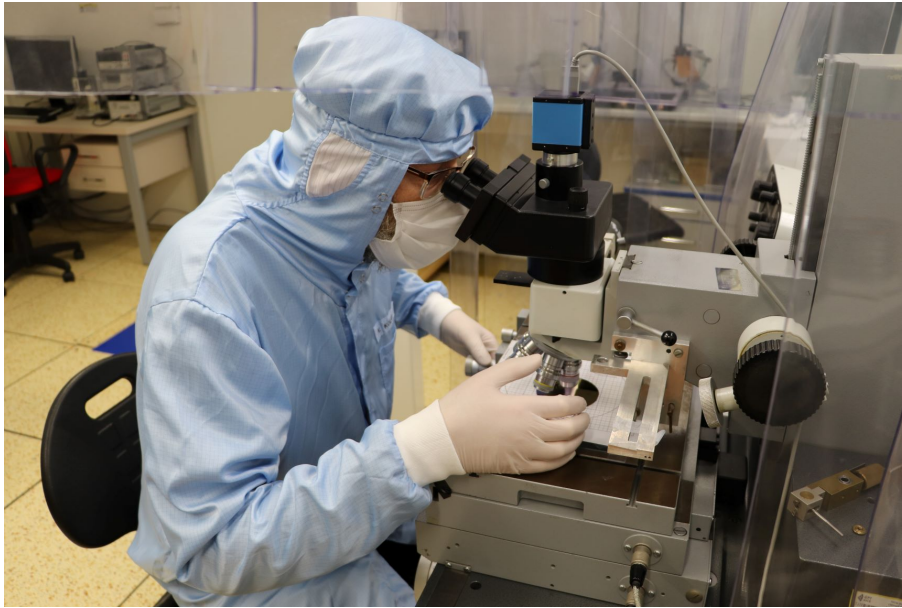
Figure 1.1: The scientist inspects defects on the wafer surface using a visible-light microscope
