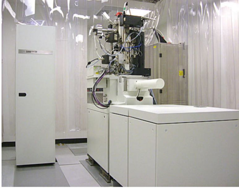
Figure 2.1: An example of electron beam lithography set up, VISTEC EBPG5000+HR at ISI CAS [15]
