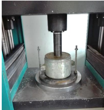
Obr. 37: IBI – penetrace trnu
