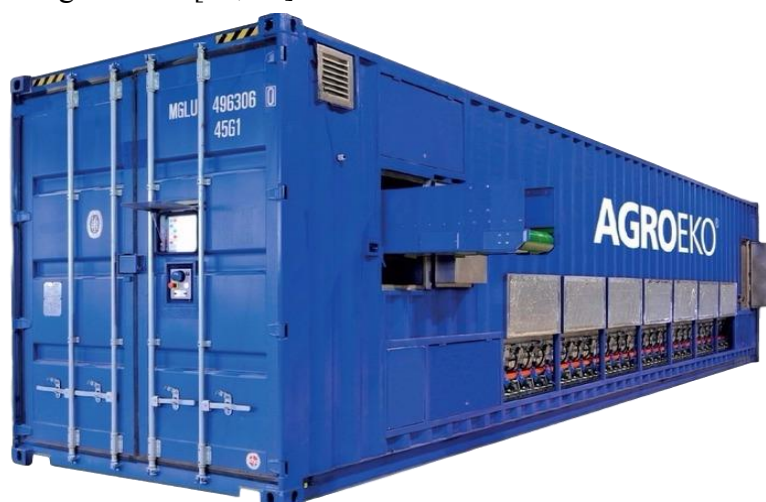
Obr. 2.1.2: Aerobní fermentor EWA (Ecological Waste Apparatus) [1]
