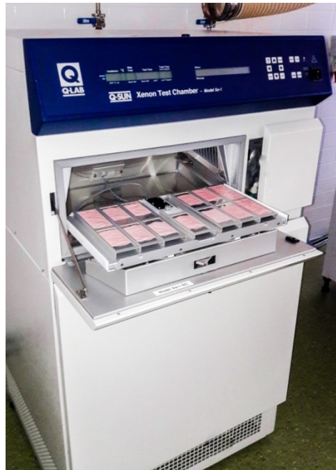
Figure 22: A photo of accelerated aging test in Q-SUN xenon chamber.
