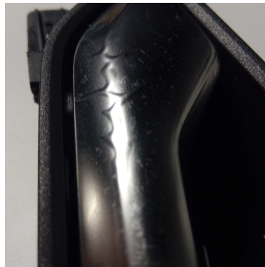
Figure 61: Separated chrome layer from handle as a consequence of often thermal changes
