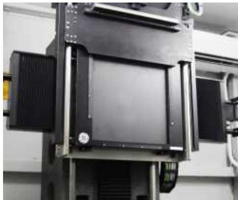
Figure 12: Flat panel detector of our GE phoenix v—tome—x L 240 tomography machine
