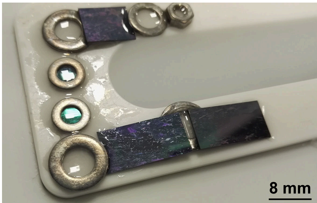
Figure 3.6: Image taken by a camera showing the deposited molecular layer on the graphene-covered substrate.
