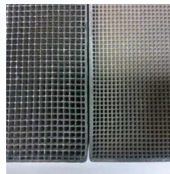
Honeycomb catalyst (100, 200 cells/in 2 )
