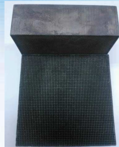
Coated on cordierite honeycomb
