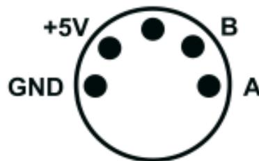
Figure 1.6: 5-pin DIN Encoder pin-out [2]
