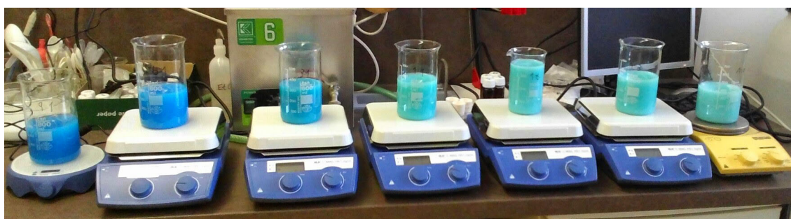
Fig. 3.10: Prepared CuO/ZnO solutions of different ratios. From the left to the right: 9:1, 6:1, 3:1, 1:1, 1:3, 1:6, and 1:9 of CuO:ZnO.
