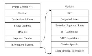
Fig. 2. Probe request structure.
