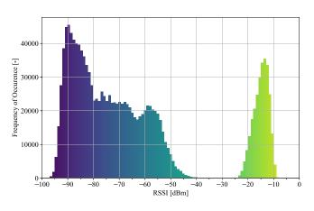
Fig. 7. Frequency of occurrence of RSSI in the captured probe requests.
