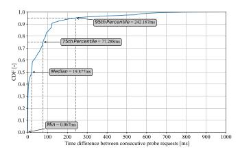
Fig. 9. CDF plot of time differences between consecutive arrivals of probe requests from the same device during a single scan.
