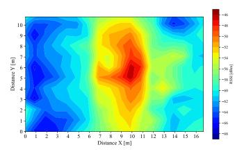
Fig. 8. RM of the RSSI in different locations of the office mapped with ESP32 microcontrollers.
