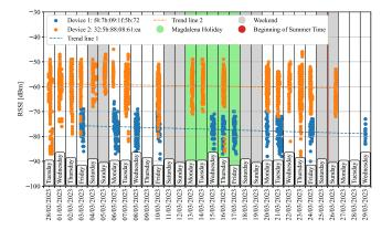
Fig. 11. Example of RSSI long-term stability evaluation for one MAC address from the dataset for two devices, both with and without MAC address randomization. (Device 1: *f4:7b:09:1f:5b:72*, device 2: *32:5b:88:08:61:ea*) including trend lines.
