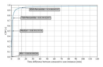
Fig. 10. CDF plot of time differences between scans of probe requests from the same device. (A time difference larger than 2 h is considered as one of the users leaving the office with the device, or turning the device OFF.)
