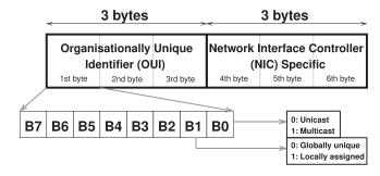
Fig. 5. Structure of MAC address with the functional bits.
