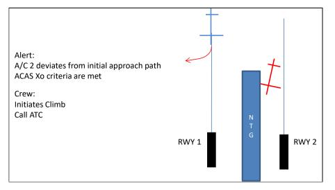
Figure 8 : Alert during CSPO-3000 approach
