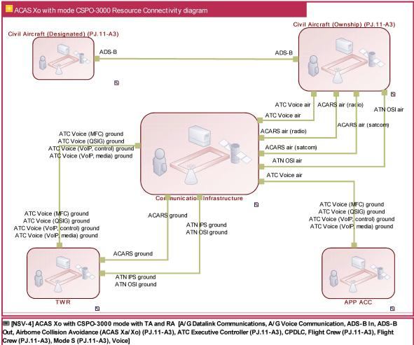
INSV-4] ACAS Xo with mode CSPO-3000 (Normal case) [A/G Voice Communication, A/G Voice Communication, ADS-B In, ADS-B Out, Airborne Collision Avoidance (ACAS Xa/Xo) (PJ.11-A3), ATC Executive Controller (PJ.11-A3), Flight Crew (PJ.11-A3), Flight Crew (PJ.11-A3), Mode S (PJ.11-A3), Tower Runway Controller (PJ.11-A3), Voice]
