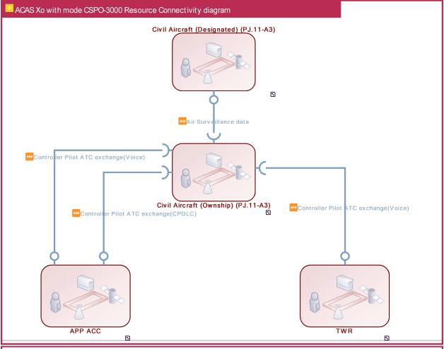
INSV-4] ACAS Xo with CSPO-3000 mode with TA and RA [A/ G Datalink Communications, A/ G Voice Communication, ADS-B In, ADS-B Out, Airborne Collision Avoidance (ACAS Xa/ Xo) (PJ.11-A3), ATC Executive Controller (PJ.11-A3), CPDLC, Flight Crew (PJ.11-A3), Flight Crew (PJ.11-A3), Mode S (PJ.11-A3), Voice]
