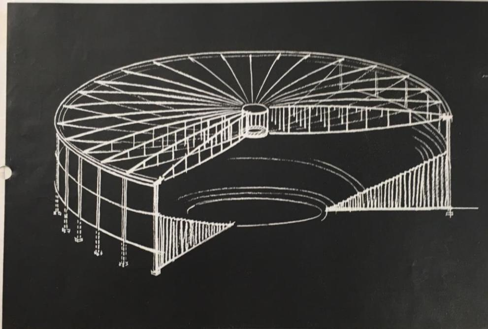
**Wheel-like roof** designed for 240'-dia. municipal auditorium in Utica, N.Y., consists of two paired layers of pretensioned cables, separated by vertical studs. The 72 cables of each layer are anchored to the inner steel tension ring and outer reinforced concrete ring which, being under constant compression, needs no expansion joint. Flutter is eliminated and unsymmetrical or upward
