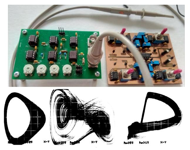
Fig. 1: Realization of chaotic oscillator having equivalent transistor cell with nonlinear forward trans-conductance (upper left), two symmetrical transistor two-ports with nonlinear both forward and backward trans-conductance (upper right), experimental evidence of structurally stable strange attractors in analyzed dynamical system (lower pictures).
