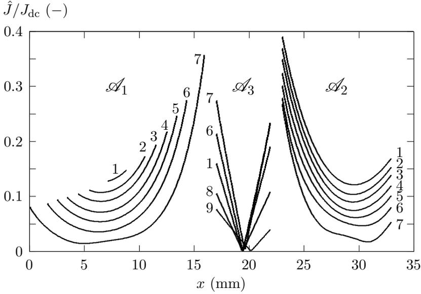
Figure 9: Variant 3: Dependence of the normed amplitude of current density on  $x$  for a constant  $y$  (expressed in mm) 1: 0.05, 2: 0.45, 3: 0.85, 4: 1.45, 5: 2.15, 6: 3.25, 7: 7.95, 8: 19.25, 9: 24.95.
