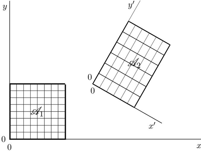
Figure 2: Example of rectangular cross sections and their approximations by aggregates in different nets of rectangles.
