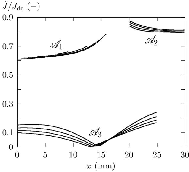
Figure 6: Variant 1: Dependence of normed amplitude of current density on  $x$  in the cross sections  $\mathcal{A}_1$ ,  $\mathcal{A}_2$  for  $y = 0.1, 1.5, 3.9, 7.9$  mm and in the cross section  $\mathcal{A}_3$  for  $y = 19.1, 20.7, 22.3, 23.9$  mm.
