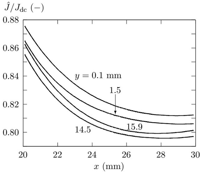
Figure 8: Variant 1: Dependence of the normed amplitude of current density on  $x$  for two pairs (0.1, 15.9) mm and (1.5, 14.5) mm of symmetrical values of  $y$  with respect to the straight line  $y = 8$  mm in the cross section  $\mathcal{A}_2$ .
