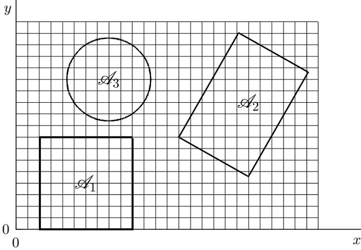
Figure 1: Cross section of conductors  $\mathcal{A}_1, \mathcal{A}_2, \mathcal{A}_3$  and net of rectangles.
