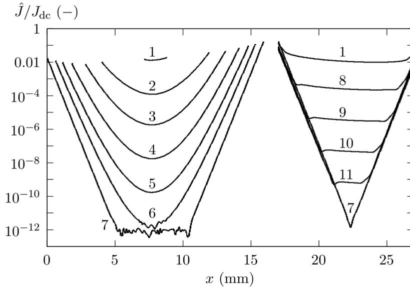
Figure 12: Variant 4: Dependence of the normed amplitude of current density on  $x$  for a constant  $y$  (expressed in mm) in the conductors  $\mathcal{A}_1$  and  $\mathcal{A}_2$ ; 1: 0.05, 2: 1.05, 3: 1.95, 4: 2.95, 5: 3.95, 6: 4.95, 7: 7.95, 8: 0.85, 9: 1.75, 10: 2.65, 11: 3.55.
