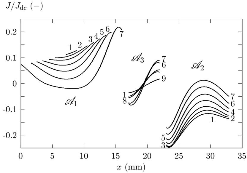
Figure 11: Variant 3: Dependence of the normed current density on  $x$  for a constant  $y$  at time  $t = 0.44917/f$ , when current in the conductor  $\mathcal{A}_1$  is at its maximum; the values  $y$  are the same as in Fig. 9 (1: 0.05, 2: 0.45, 3: 0.85, 4: 1.45, 5: 2.15, 6: 3.25, 7: 7.95, 8: 19.25, 9: 24.95).
