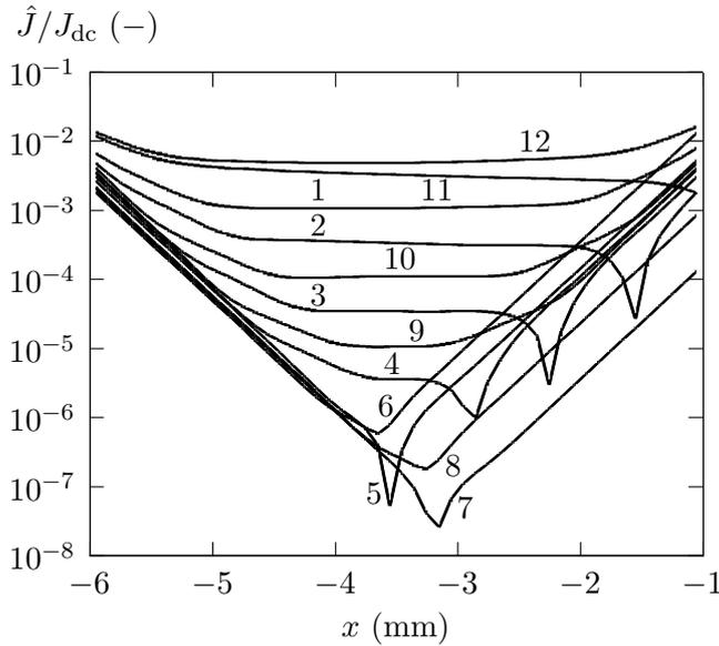
Figure 13: Variant 4: Dependence of the normed amplitude of current density on  $x$  for a constant  $y$  (expressed in mm) in the conductor  $\mathcal{A}_3$ ; 1: 0.05, 2: 0.65, 3: 1.25, 4: 1.85, 5: 2.65, 6: 7.95, 7: 18.95, 8: 19.95, 9: 23.35, 10: 23.95, 11: 24.55, 12: 24.95.
