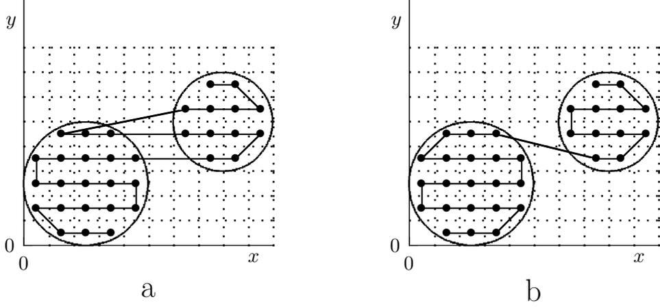
Figure 3: Example of two path graphs in the loop of two cylindrical conductors. Dotted line segments represent the net of rectangles, the centres of partial conductor cross sections, i.e. graph vertices are designated by  $\bullet$ , the line segments connecting the graph vertices are its edges.
