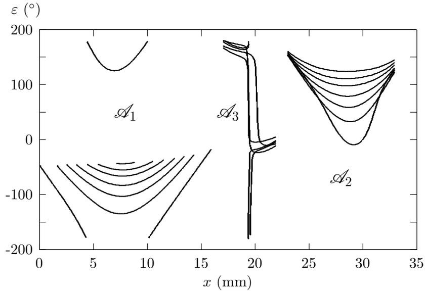
Figure 10: Variant 3: Dependence of the initial phase of current density on  $x$  for a constant  $y$ ; the values  $y$  are the same as in Fig. 9 (1: 0.05, 2: 0.45, 3: 0.85, 4: 1.45, 5: 2.15, 6: 3.25, 7: 7.95, 8: 19.25, 9: 24.95).
