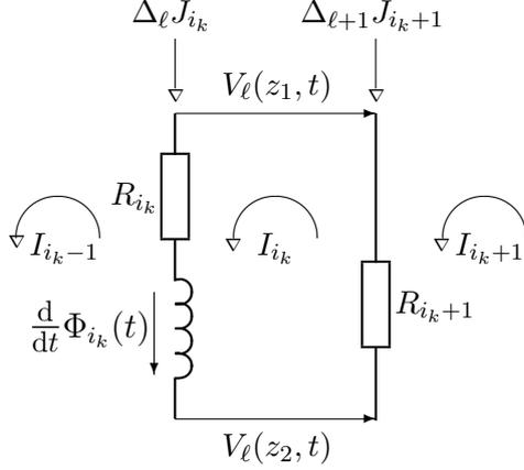
Figure 4: The equivalent circuit of the  $i_k$ th partial loop segment between the planes  $z = z_1$  and  $z = z_2$  in the case of (4).
