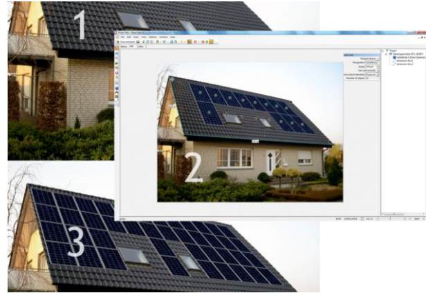
Figure 4: Students also learn how to work with Photo plan, integrated into the PV*SOL environment for a realistic representation of future photovoltaic systems.
