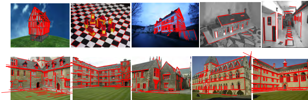
Figure 7: Camera pose estimation from line correspondences. The images are overlaid with reprojections of 3D line segments using the camera pose estimated by the our method DLT-Combined-Lines .
