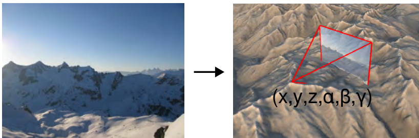
Figure 2: The goal of visual geo-localization is to determine the position (x, y, z) of the camera (right) that captured the query image (left). Camera orientation estimation methods focus on calculating the camera’s rotation angles (\alpha, \beta, \gamma) .
