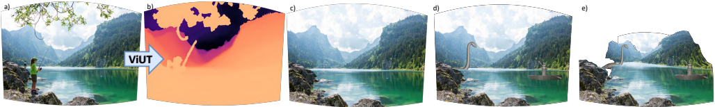
Figure 25: ViUT depth estimation: our model uses input RGB image (a) to estimate its absolute depth (b). The resulting map can then be used for further applications, such as object removal (c), 3D scene manipulation (d), or scene reconstruction (e).
