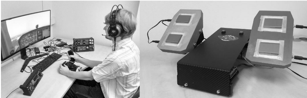
Figure 10: Flight simulator setup on the left side with rudder pedal detail on the right side [29]
