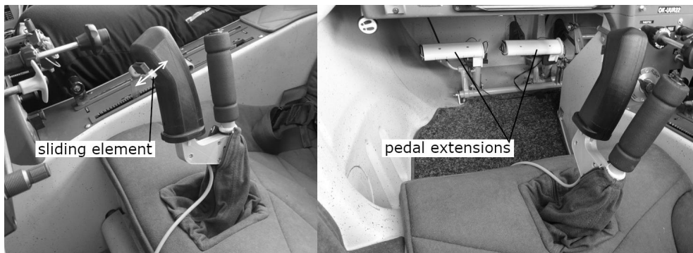
Figure 11: Sliding element and vibration pedals mounted in the aircraft cockpit [29]
