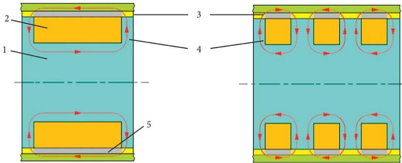
Figure 10: Single-coil structure (left); three-coil structure (right): 1, magnetic circuit; 2, electromagnetic coil; 3, annular gap; 4, magnetic flux lines; 5, non-magnetic section [46]
