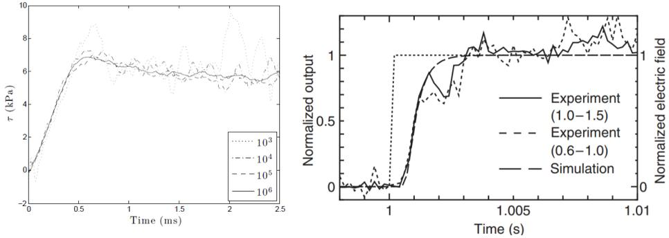
Figure 5: The time dependency of shear stress on step change of control signal from Sherman model (left) [34] and Koyanagi experiments (right) [37]
