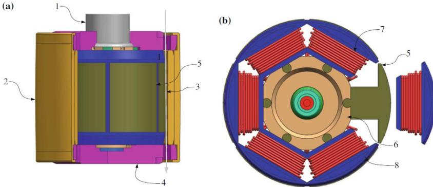
Figure 14: MR control valve with laminated magnetic circuit: 1, rod; 2, sleeve; 3, annulus gap; 4, lids; 5, magnetic poles; 6, coil core; 7, electromagnetic coil; 8, casing [6]
