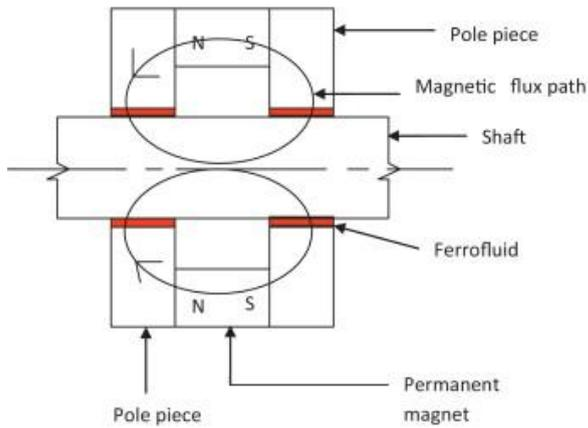
Figure 12: Conventional design of seal with magnetic fluid [47]
