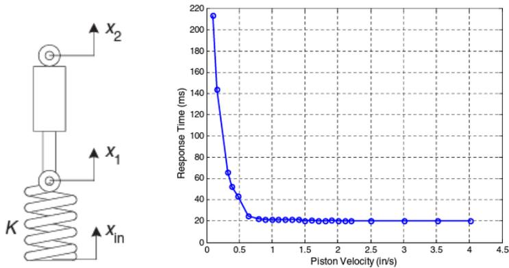
Figure 15: The effect of piston velocity on MR damper response time [54]
