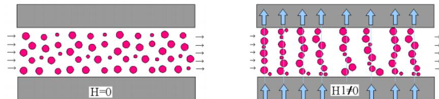
Figure 2: Magnetorheological effect; left: without the magnetic field, right: with the application of magnetic field (blue arrow)[11]
