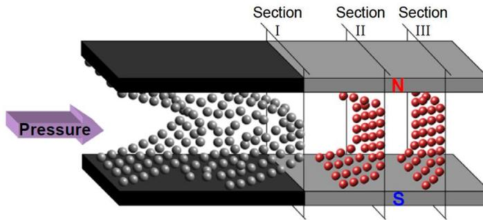
Figure 6: Velocity profile development of MR fluid under magnetic field [41]
