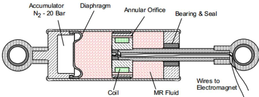
Figure 9: Mono-tube magnetorheological damper [18]
