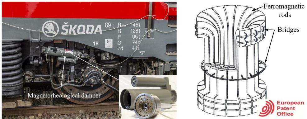
Figure 16: Developed MR damper with short response time mounted on locomotive Škoda Transportation during testing (left), the main idea of structured magnetic circuit patent (right)
