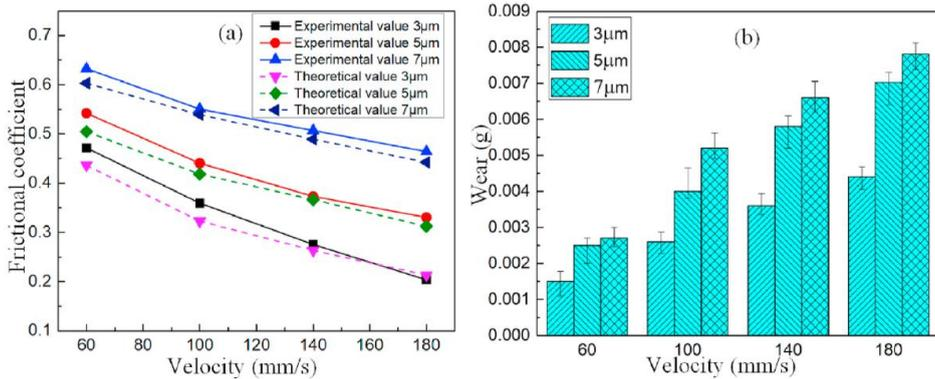
Figure 3: The effect of particle size on friction coefficient and wear for O-ring seal flooded in MR fluid [26]
