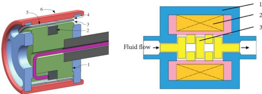
Figure 11: Dual-gap piston structure (left)[6]: 1, core coil; 2, electromagnetic coil; 3, gap 1; 4, gap 2; 5, non-magnetic spacer; 6, sleeve; meandering valve (right) [46]: 1, magnetic circuit; 2, electromagnetic coil; 3, meandering path
