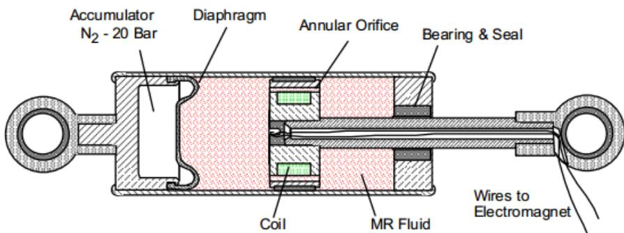
Figure 9: Mono-tube magnetorheological damper [18]
