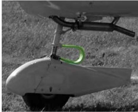
Figure 4.9: Nose gear spring on the airplane.
