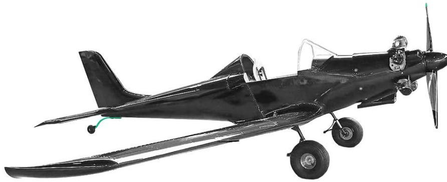
Figure 5.2: Tail gear spring (in green): Merlin Sportster. Courtesy of TechProAviation, s.r.o.
