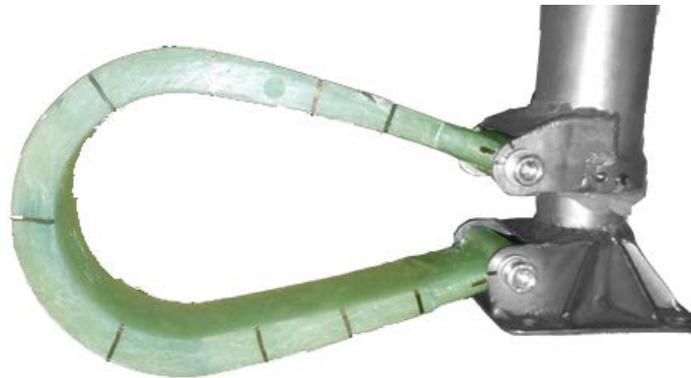
Figure 4.12: Spring in the test jig with control marks.
