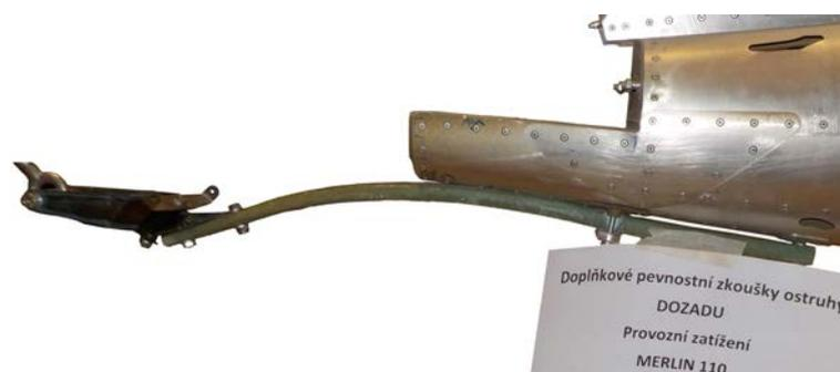
Figure 4.14: Supplementary condition up + aft - limit load.
