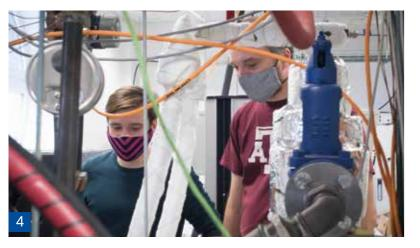
Karel Katovsky from the Department of Electrical Power Engineering of the Faculty of Electrical Engineering and Communication presents an experimental loop that allows simulation of the reaction to a sharp temperature rise in a nuclear reactor.
