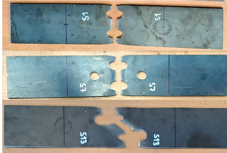
Figure 3.9: Photographs of ruptured plates with centered and staggered bolt holes
