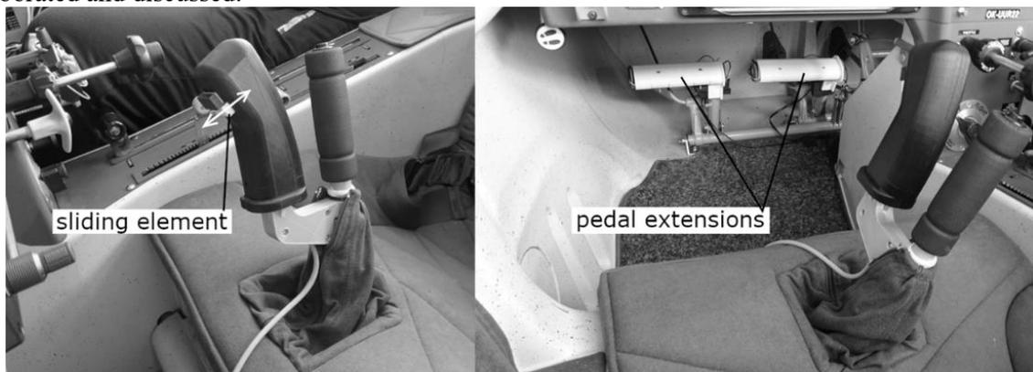
**Figure 2** Hardware conveying AoA and AoS to a pilot through haptic feedback [4]
