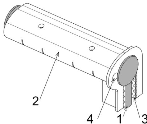
Figure 9: A sample solution of rod-type pedal with vibration motors position (**Hab-7**)
