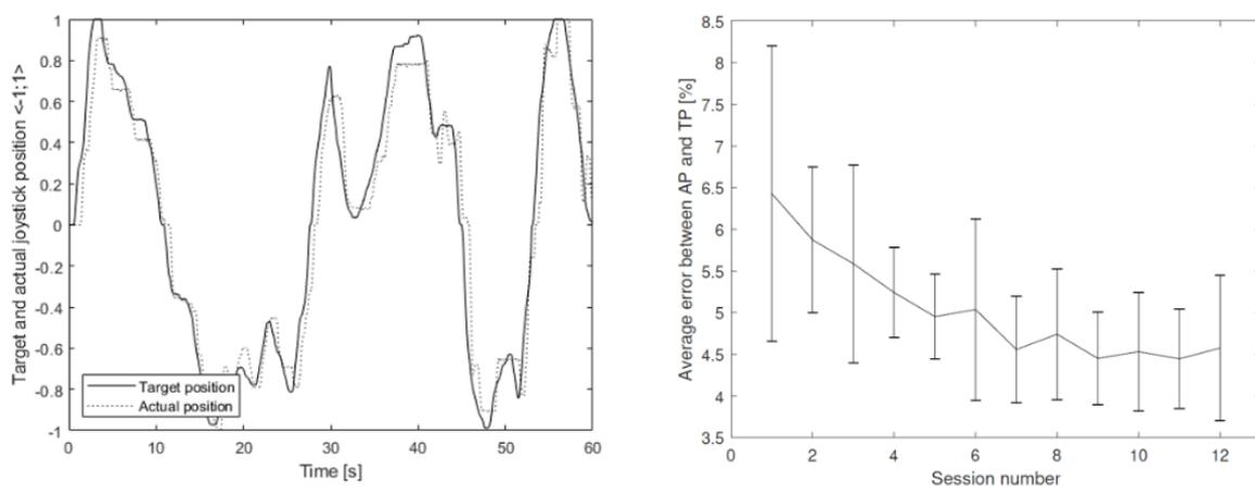
**Figure 3** Results obtained in a haptic guidance task without visual assistance. On the left side, a sample task displays the target and actual joystick positions. On the right side, the graph illustrates the mean error between target and actual positions for all participants along sessions.
