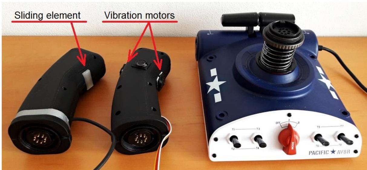
Figure 3: Sliding element and vibration motors joystick handles (**Hab-3**)
