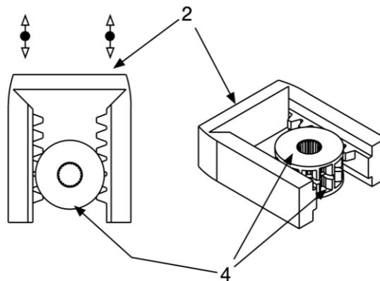
Figure 7: Sliding element gearing mechanism which allows symmetrical and asymmetrical movement (**Hab-6**)
