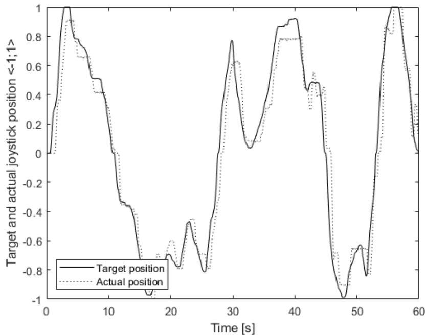
Figure 5: Sample recording of the guidance to continuously changed forward to backward joystick position tested in Task 2 (**Hab-9**)
