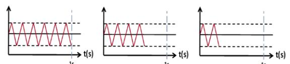
Figure 4: Example of signal's changing duration
