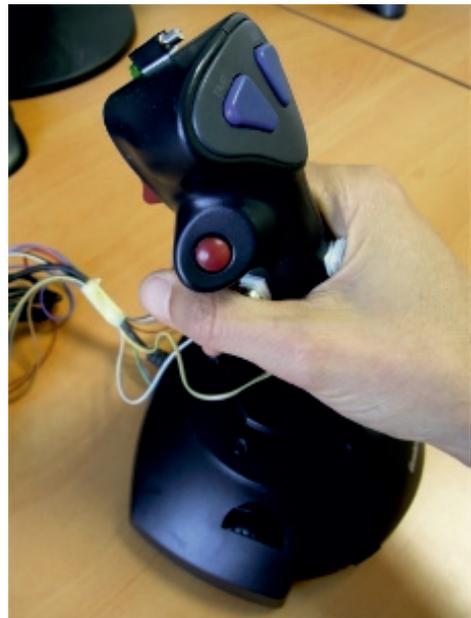
Figure 1. Joystick with vibration motors.
