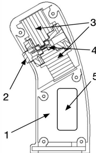
Figure 6: Joystick handle with two servos powering the sliding element (**Hab-6**)
