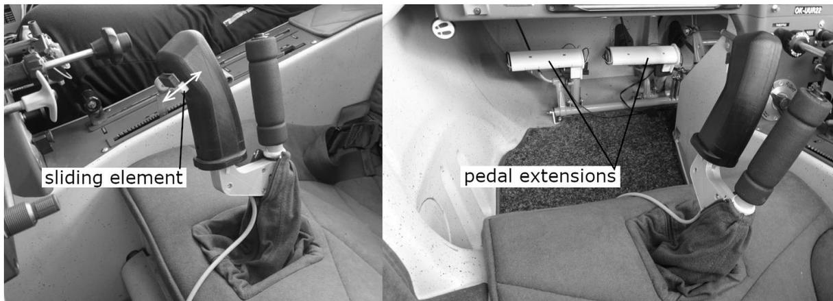
Figure 11: Sliding element and vibration pedals mounted in the aircraft cockpit (*Hab-8*)
