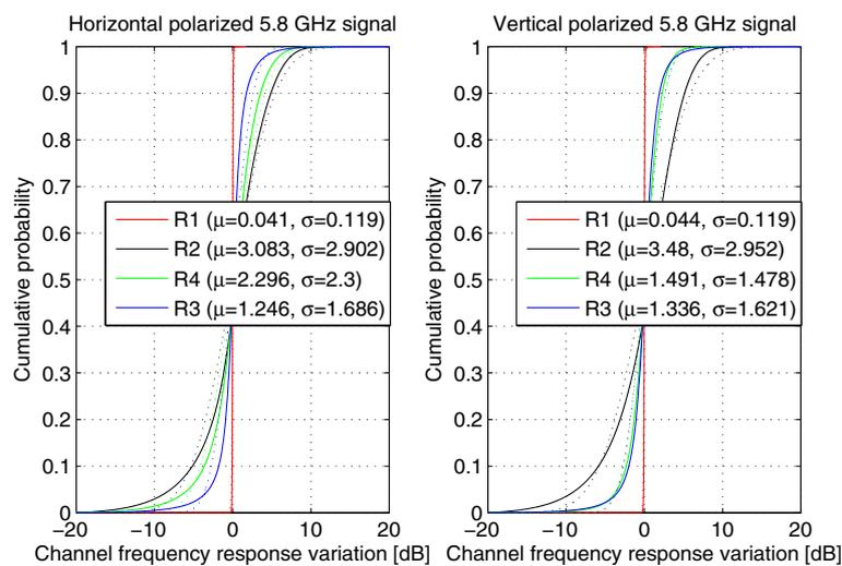
**Fig. 15** Cumulative distribution function of channel frequency response variation of 5.8 GHz center frequency for both horizontal and vertical co-polarization. The curve colored in red, black, blue, and green represent the calculated channel frequency response variation for the first to the fourth routes, respectively. The colored dotted lines represent the normal distribution of the corresponding measured channel frequency response variation values
