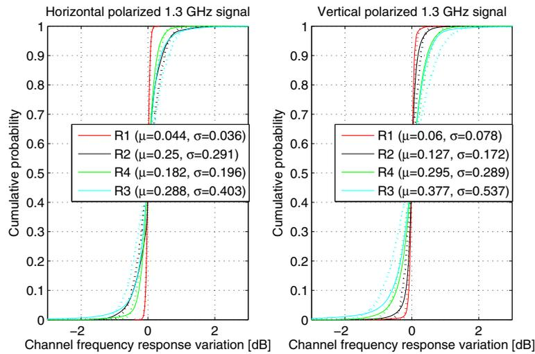
**Fig. 14** Cumulative distribution function of channel frequency response variation of 1.3 GHz center frequency for both horizontal and vertical co-polarizations. The curve colored in red, black, blue, and green represent the calculated channel frequency response variation for the first to the fourth routes, respectively. The colored dotted lines represent the normal distribution of the corresponding measured channel frequency response variation values
