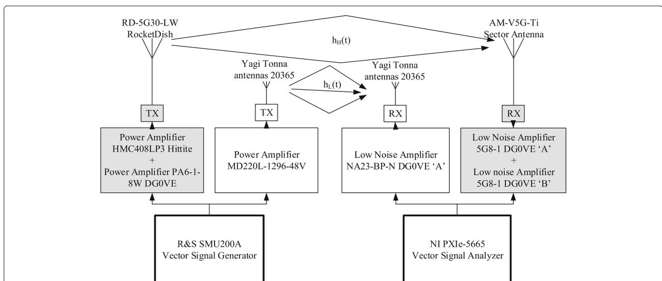
**Fig. 3** Channel sounder setup. Channel sounding systems diagram with transmitter and receiver for both ultra high frequency (white colored) and super high frequency (gray colored) bands
