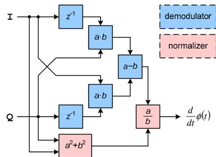
Fig. 7. Delay-multiply FSK demodulator
