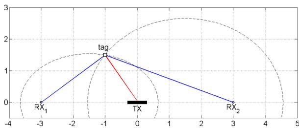
Figure 1. Localization using ellipses intersection in a MISO system.
