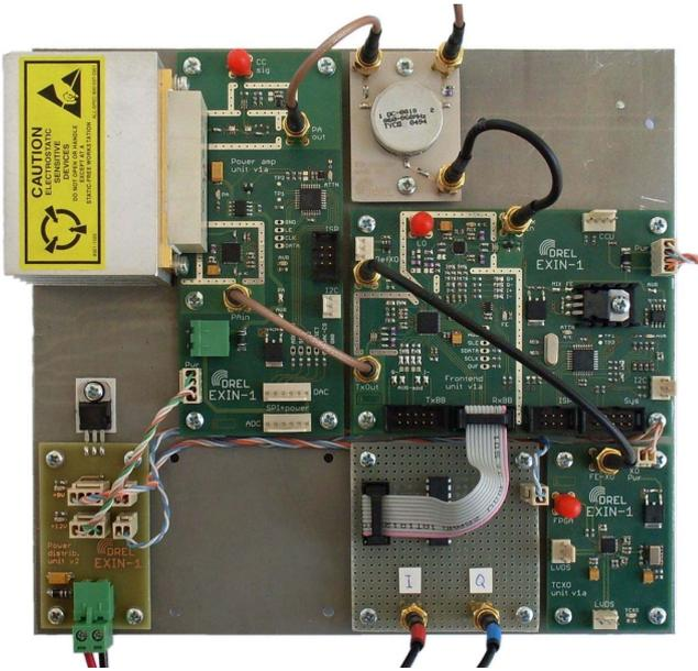
Figure 4. Experimental UHF RFID front-end.
