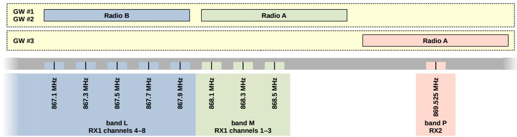
Figure 1. LoRaWAN EU868 channels and sniffer front ends.
