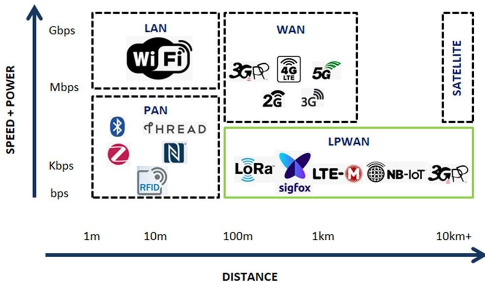
Fig. 3.1: LPWAN compared with the other existing technologies [24].
