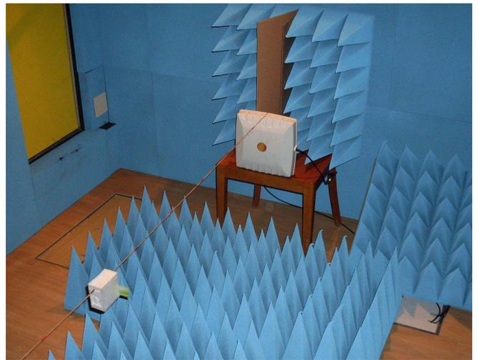
Figure 2. Measurement setup in an RF anechoic chamber.
