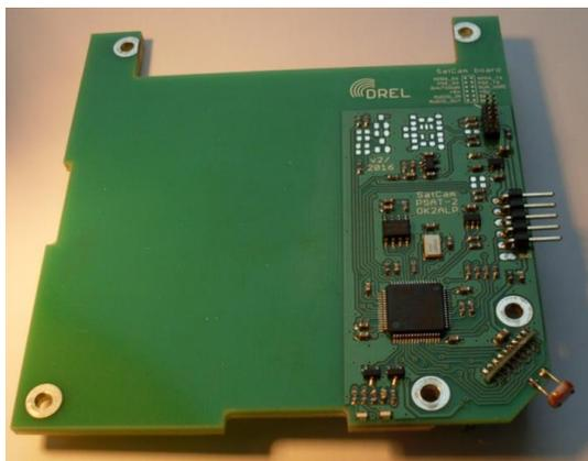
Obr.1 Camera control board
