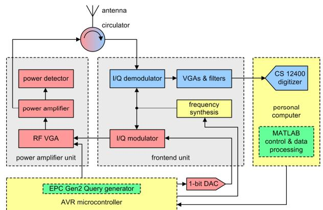
Figure 3. Block diagram of the measurement system.
