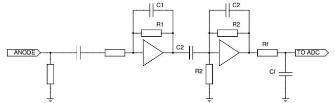
**Fig. 3.** Block-level schematics of the analog signal chain between the MPPC output and the ADC. This two-stage amplifier is formed by a traditional charge sensitive amplifier with  $R_1 C_1 = 3.3$  ms decay constant and an RC-CR shaping amplifier  $\tau = 2.2$   $\mu$ s.
