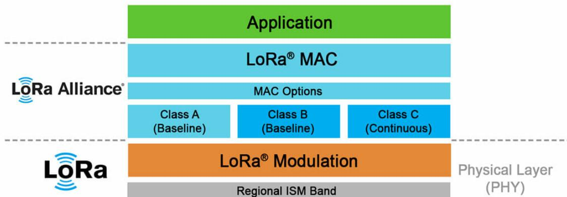
Fig. 3.2: Physical and Communication layers of a LoRaWAN Network [28].
