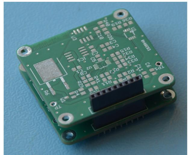
Fig. 20. PQ9 PocketQube boards with stackable pin connector.
