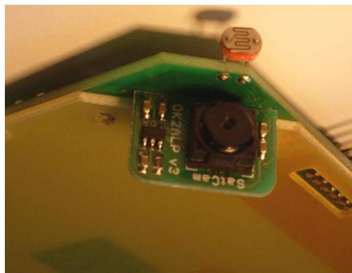
Obr.2 Position of camera module
