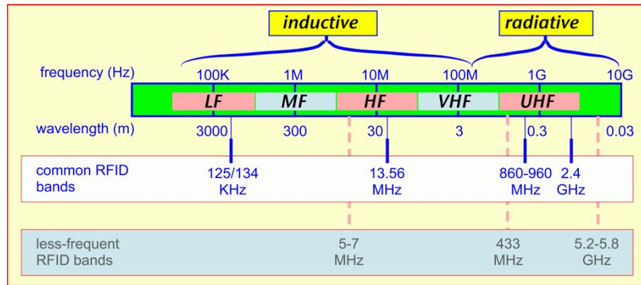
Fig. 2.1: Overview of RFID communication bands with coupling type [1].
