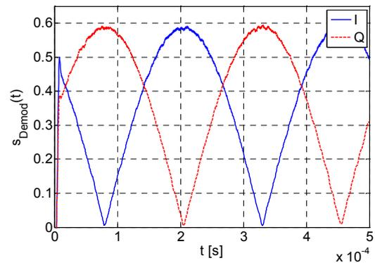
Fig. 3. I and Q signals after AM demodulation
