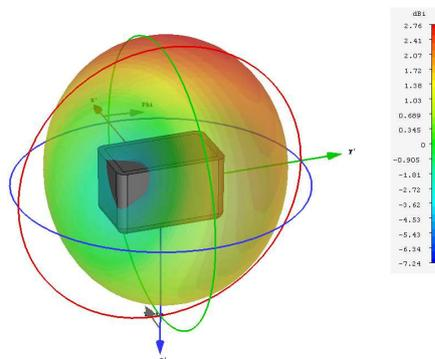
Fig. 2: Antenna simulation at 2.4GHz
