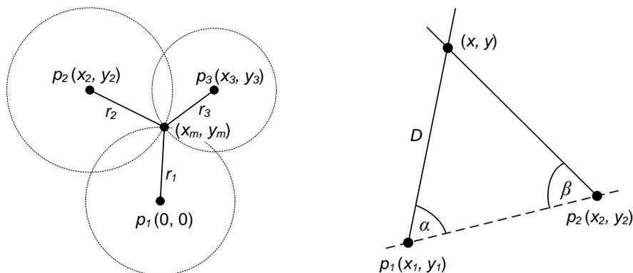
Fig. 2.6: Trilateration and triangulation positioning [12].
