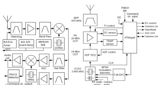
Obr.1 Transponder block diagram
