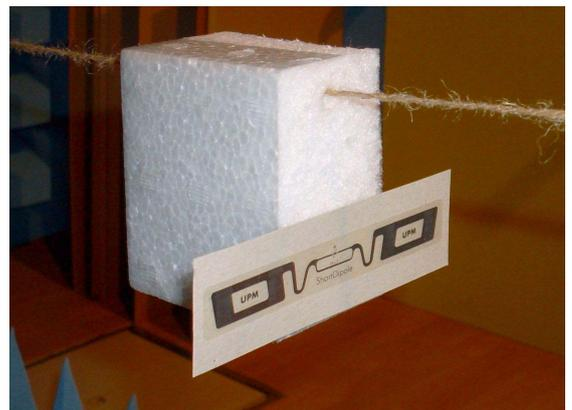
Figure 6. UPM ShortDipole<sup>x</sup> tag mounted on a positionable holder.
