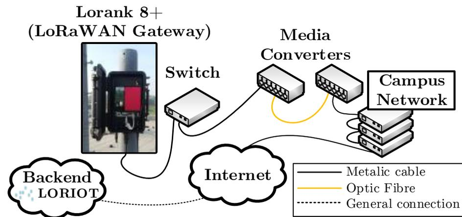
Figure 5. Topology of our LoRaWAN experimental single-gateway network.
