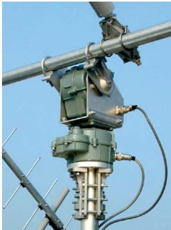
Fig. 4.6: Azimuth-elevation rotator.
