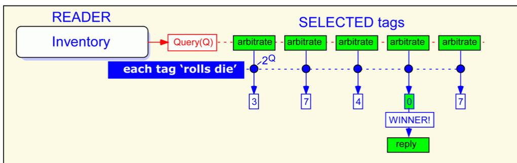
Fig. 2.3: Structure of the EPC Gen2 “Query” command [1].
