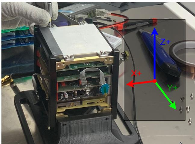
**Fig. 5.** Stack of GRBAlpha and the reference frame with respect to the satellite. From top to bottom: chasing of the gamma detector, gamma detector payload electronics (see also Fig. 2), onboard computer and GNSS receiver, sensor board, power supply, radio transceivers, and antenna deployer.
