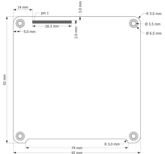
Fig. 19. CS14 printed circuit board outline.
