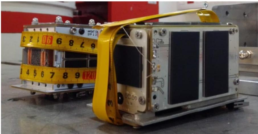
Fig. 4.3: Antennas from a tape measure on the HADES satellite.
