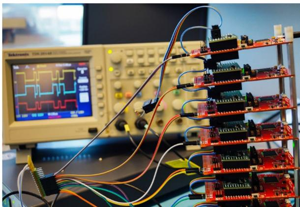
Fig. 4. Test setup for data bus characterization.
