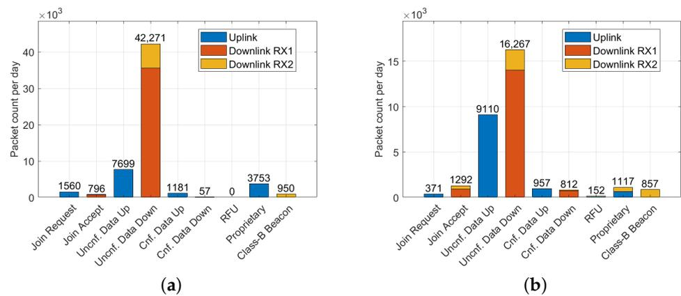
**Figure 5.** LoRaWAN message types: Join Request, Join Accept, Unconfirmed/Confirmed Data Up/Down, RFU, Proprietary, and Class-B Beacon in: (a) Vienna dataset; (b) Brno dataset.
