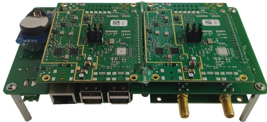
**Figure 3.** Photo of the LoRaWAN sniffer internal hardware.
