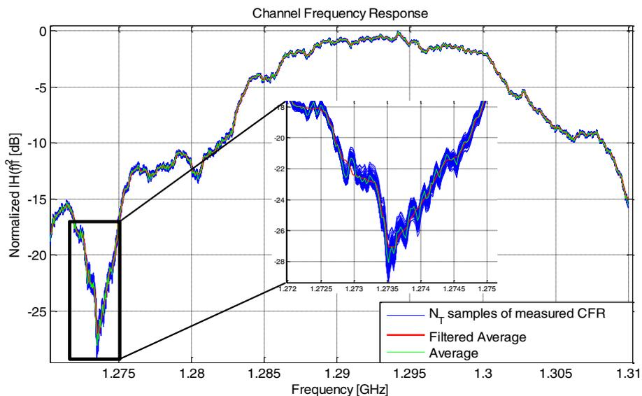
**Fig. 5** Normalized  $|H(f)|^2$  used to characterize the channel frequency response. The blue curve represents  $N_T$  measured channel frequency response during 8 s. The green curve represents the average value of the measured channel responses. The red curve depicts the smoothed version of channel frequency response after applying the median filter
