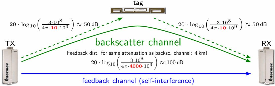
Fig. 2.2: Signal propagation in a degenerated RFID channel [1]. The red numbers correspond to distance in the path loss formula, i.e. a backscatter channel with a distance of 20 m has a similar attenuation as a 4 km feedback channel.
