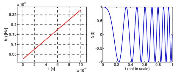
Fig. 1. Linear chirp signal
