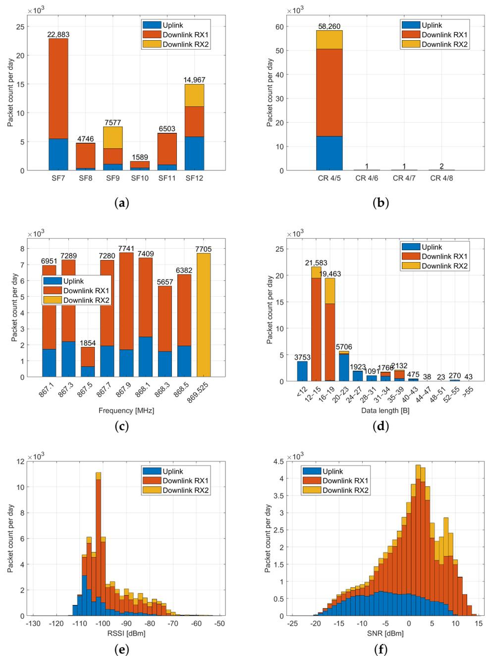
**Figure 6.** Parameters of captured LoRaWAN messages in the Vienna dataset: (a) Spreading factor; (b) Coding ratio; (c) Channel occupation; (d) Payload length; (e) Received Signal Strength Indicator (RSSI); (f) Signal-to-Noise Ratio (SNR).
