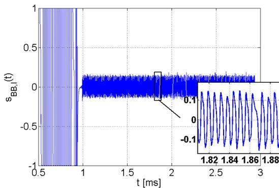
Figure 8. In-phase baseband signal received from the tag.
