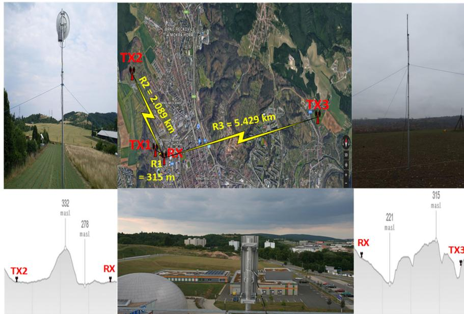
**Fig. 1** Measurement locations for R1, R2, and R3 routes. Line of sight route R1 = 315 m and non-line of sight route R2 = 2.089 km with super high frequency band TX2 position on the left-hand side, R3= 5.429 km with ultra high frequency band TX3 position on the right-hand side and the position of the sector receiver antenna used for the super high frequency signal of TX2-RX measurements. Map source: Google.com, Mapy.cz
