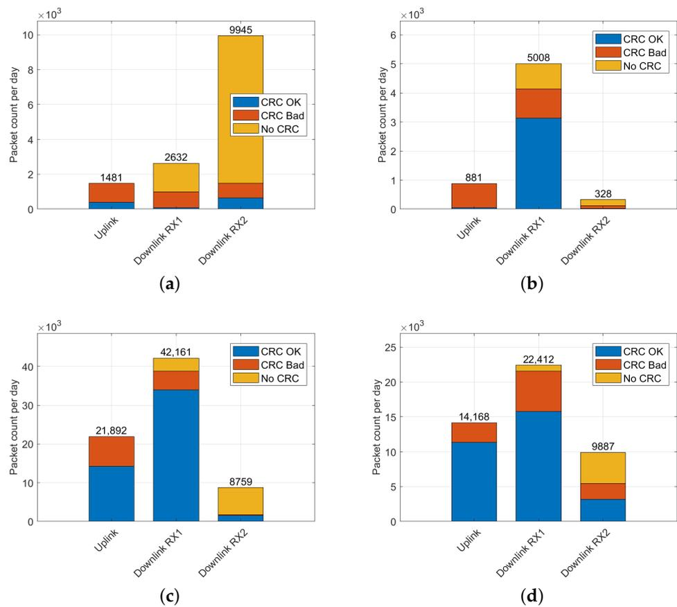
**Figure 4.** Distribution of LoRaWAN packets for individual receive chains for packets with valid, invalid, and missing CRC in: (a) Liege dataset; (b) Graz dataset; (c) Vienna dataset; (d) Brno dataset.
