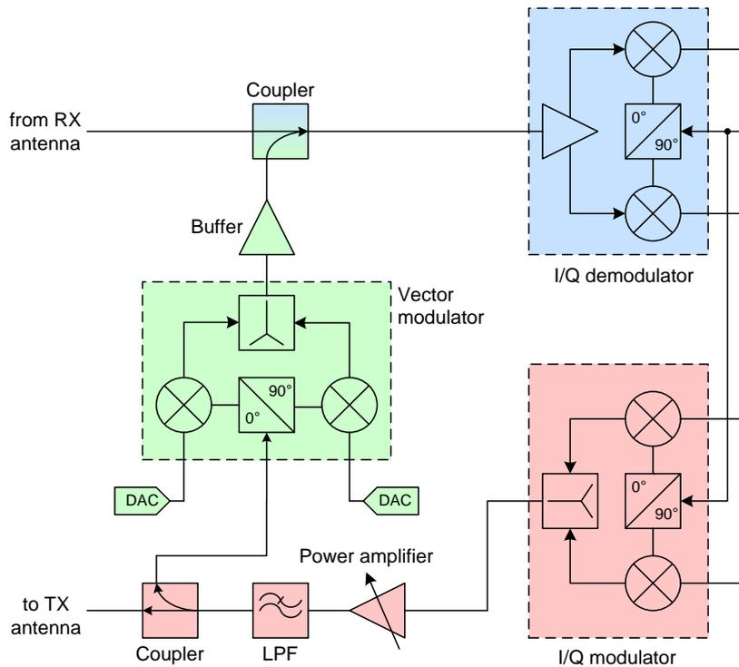
Fig. 2.5: Carrier cancellation by a destructive interference integrated in an SDR [12].
