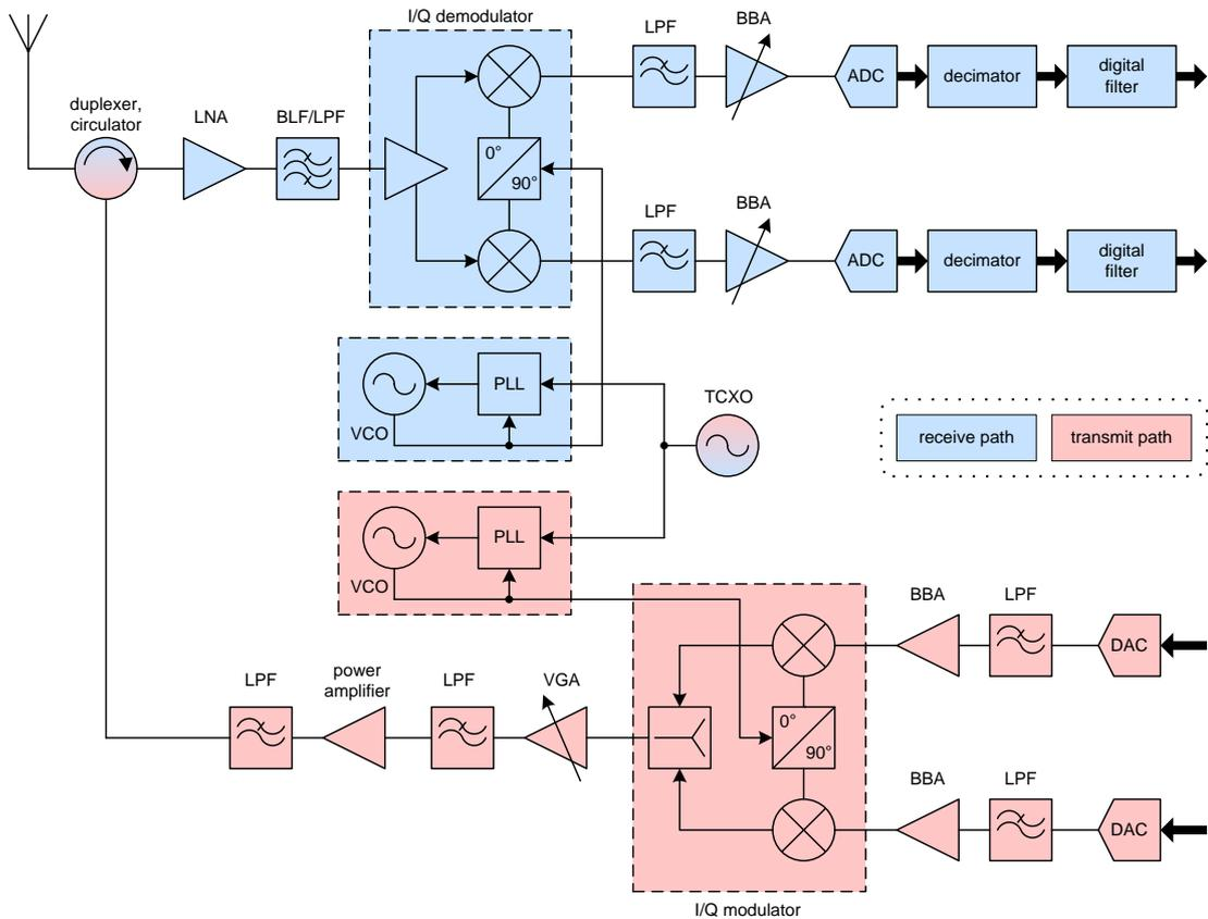
Fig. 2.4: I/Q transceiver architecture for a software-defined radio [12].
