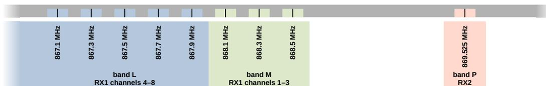
Fig. 3.3: LoRaWAN EU868 channels [31].
