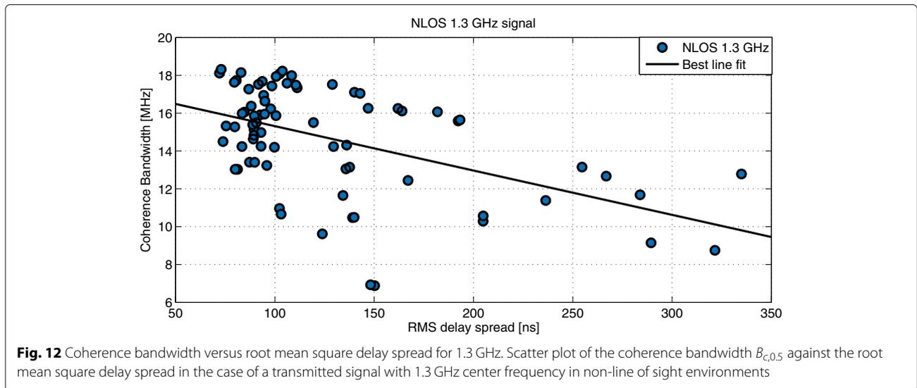
transmitter and a transmitter at 1.3 GHz and a parabolic RD-5G30-LW RocketDish antenna transmitter and AM-V5G-Ti sector antenna receiver at 5.8 GHz. The vertical and the horizontal co-polarizations were presented in both line of sight and non-line of sight scenarios. As output, channel characteristics such as root mean square delay spread, path loss, coherence bandwidth, and channel frequency response variation were extracted.
