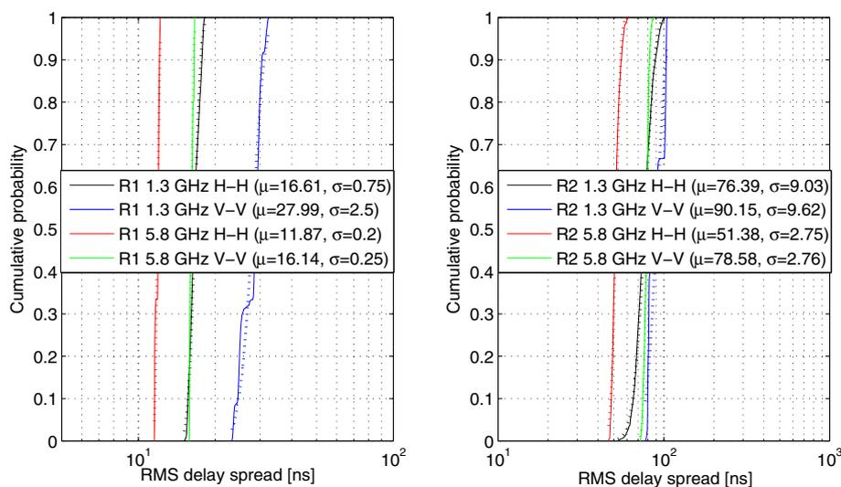
**Fig. 9** R1 and R2 root mean square delay spread. Cumulative Distribution Function of the root mean square delay spread in [ns] for different frequencies and both horizontal and vertical co-polarizations of the first and second measurement routes (R1 and R2) in line of sight and non-line of sight scenarios, respectively. The colored dotted lines represent the Normal distribution of the corresponding frequency and polarization combinations
