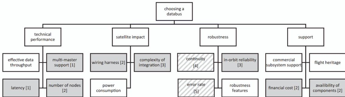
Fig. 4.5: Derivation tree for nanosatellite bus selection [53].
