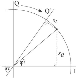
Figure 7. Phase imbalance correction.
