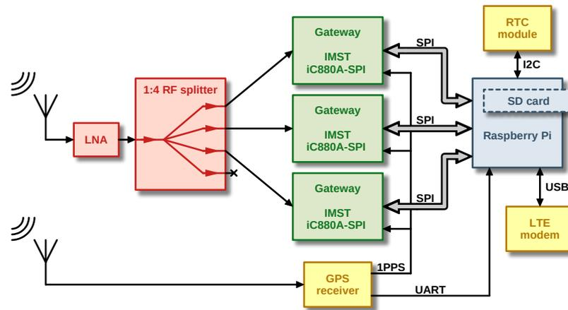
Figure 2. Block diagram of the developed LoRaWAN sniffer.
