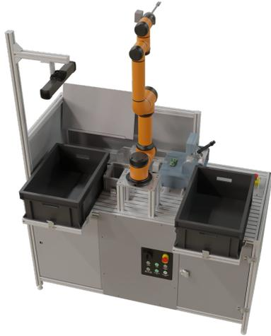
(a) Render of a PCB testing workplace with the Ensenso 3D camera for bin-picking, 6 DoF Aubo i5 robot, 2 DoF custom-build robot, functional tester, barcode reader, and printer, source, and target boxes.
