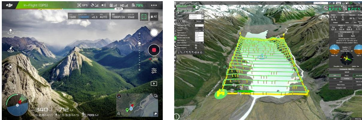
(a) GUI with first-person view and sensory data from flying drone<sup>16</sup>.
