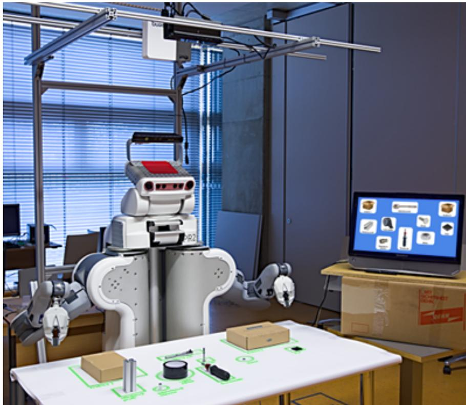
Figure 13: Prototype of the human-robot shared-space environment with augmented reality user interface (Materna et al., 2016).
