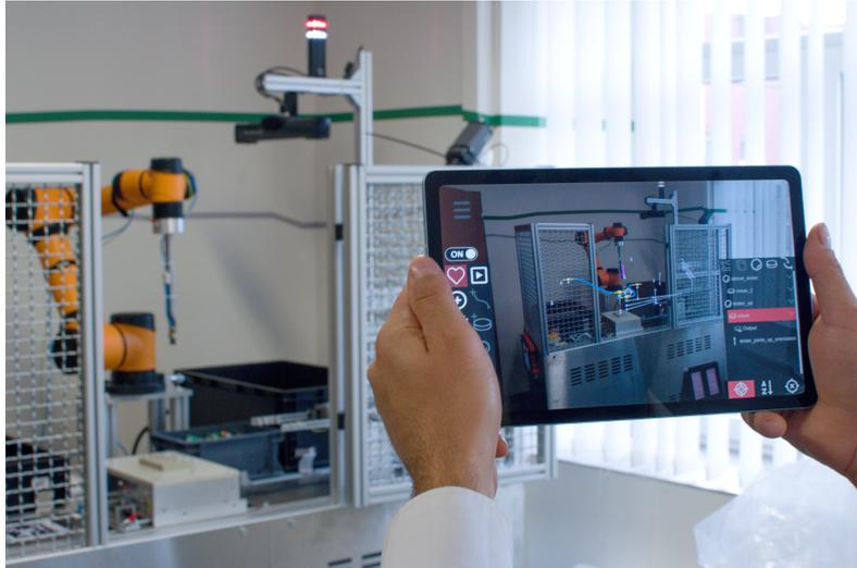
(a) Robot-operator observing the program for the PDB testing task in augmented reality (Kapinus et al., 2022c).
