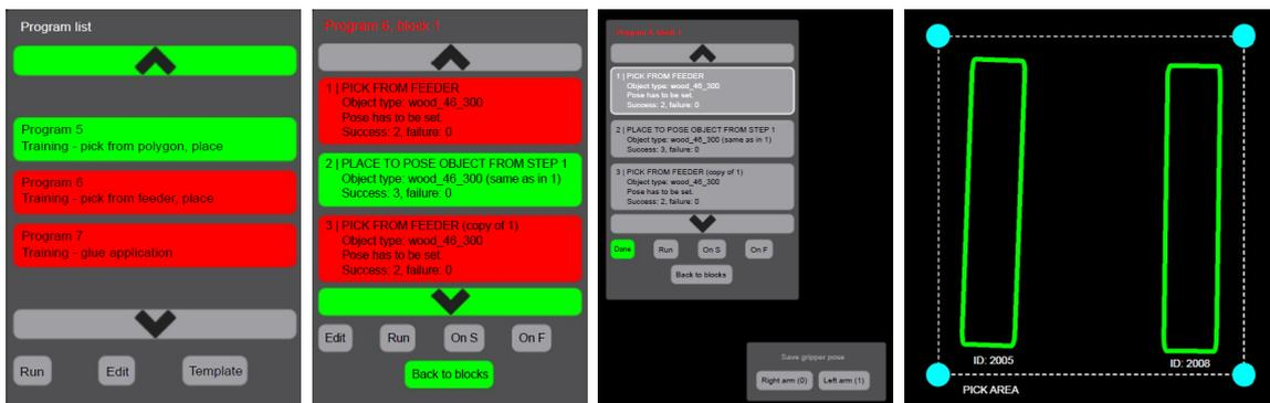
(a) List of programs. (b) List of instructions. Green ones are ready to run, red ones need to set parameters. (c) A small dialog shows if the robot is able to detect an object in the feeder up. The green outlines and allows the user to respond to detected objects. (d) Polygon defining the area from which the robot on the table from which the objects will be picked. The green outlines and allows the user to respond to detected objects. (e) Save the arm pose.
