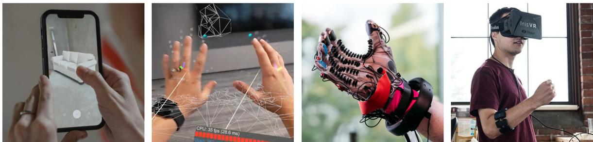
Figure 4: Examples of user-input technologies (from left to right): surface gestures e.g. on mobile devices<sup>8</sup>, free-space gestures e.g. by HoloLens<sup>9</sup>, VR gloves e.g. Meta prototype<sup>10</sup> and wearable sensors e.g. Myo Armband<sup>11</sup>.
