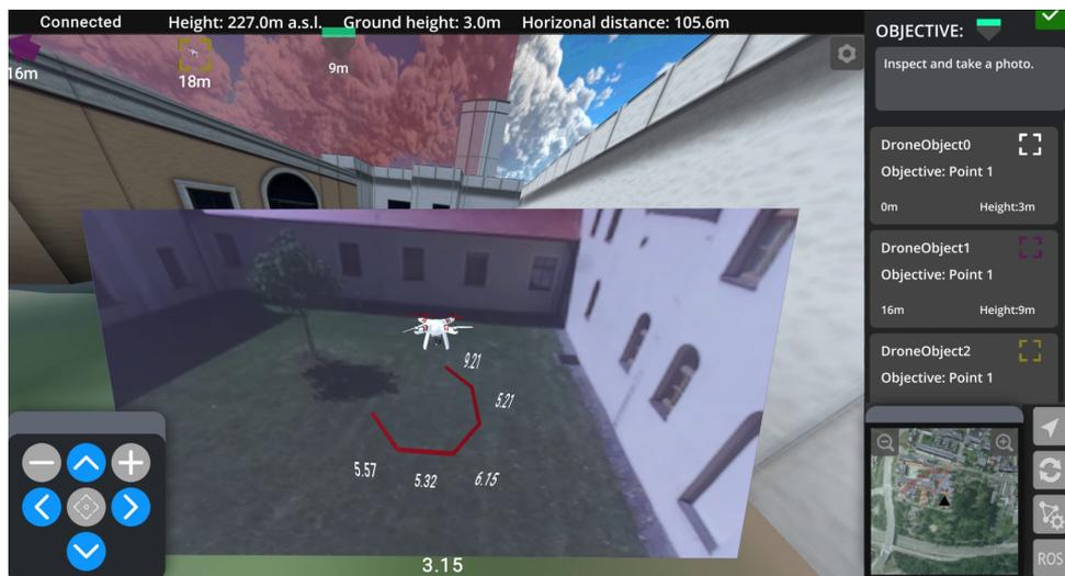
(b) Drone pilot GUI application based on augmented virtuality (DroCo)<sup>1</sup>.
