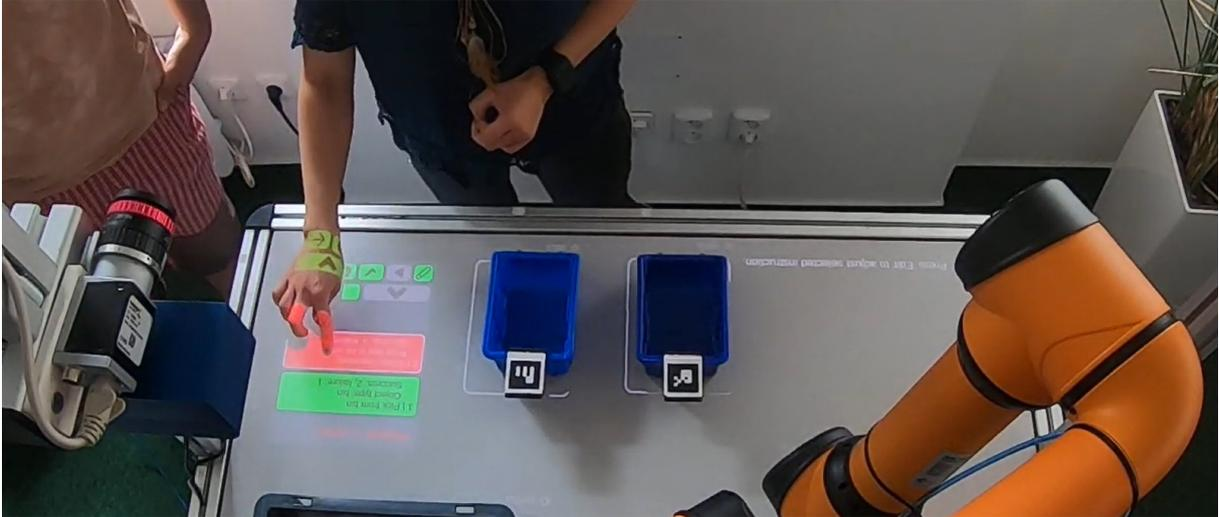
Figure 18: Participant programs a visual inspection task using the proposed spatial augmented reality interface (Kapinus et al., 2020).
