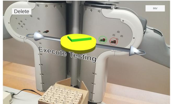
Fig. 5. The *puck* consists of central disc, two circles representing the input and the output and two pipes connecting input/output with the disc. In the first prototype, the type of the *puck* is represented by its color and the text placed in front of the disk. Above the pipes, small 3D models of input and output workpieces are placed.
