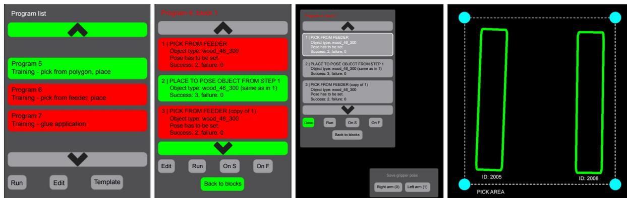
(a) List of programs. Green ones are ready to run, red ones need to set parameters. (b) List of instructions. Green ones are ready to run, red ones need to set parameters. (c) A small dialog shows if the robot is able to detect an object in the feeder and allows the user to save the arm pose. (d) Polygon defining the area on the table from which the objects will be picked up. The green outlines correspond to detected objects.
