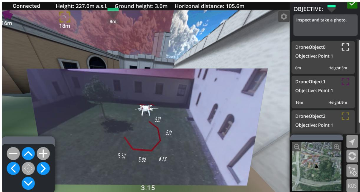
Figure 29: Screenshot from an application with GUI (DroCo) using augmented reality to implement a third-person view with live transmission of real video-data and GUI elements visualising estimated distances to virtual objects.
