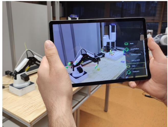
Fig. 1. A user observes the scene with robotic program visualized in AR. There is a crosshair and side menu for indirect object selection.
