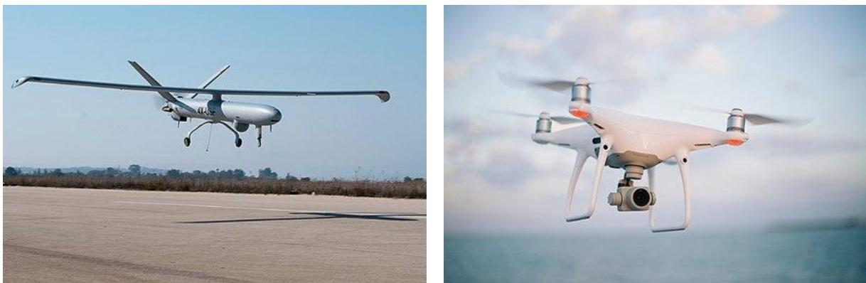
Figure 9: Examples of typical UAVs: fixed-wing UAV (left) and quadrotor UAV (right).
