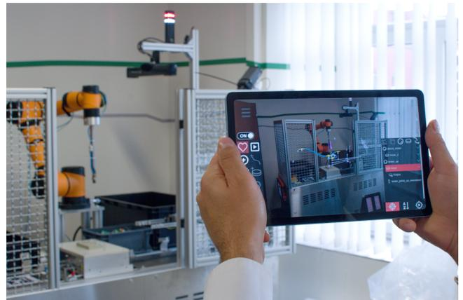
Fig. 1: A user observes the program for the PCB testing task through the tablet.
