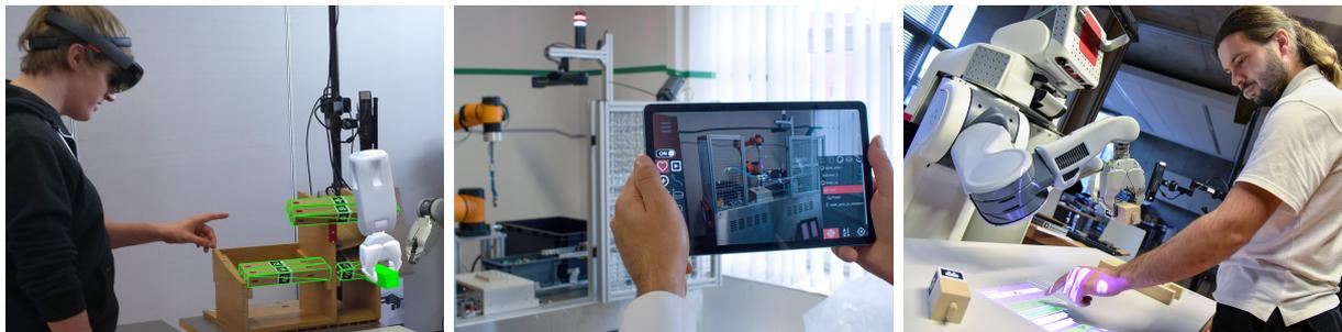
Figure 3: Examples of augmented reality visualisation technologies (from left to right): head-mounted display (Microsoft HoloLens), mobile device and projected AR.
