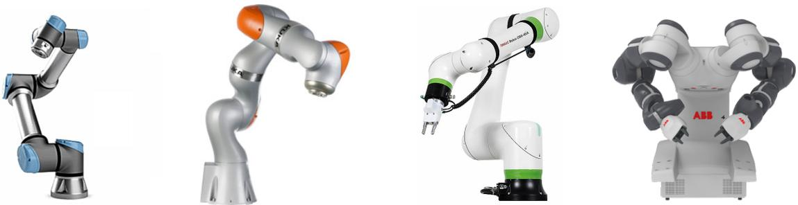
Figure 5: Examples of collaborative robots (from left to right): Universal Robots (UR), KUKA, FANUC a ABB Yumi.
