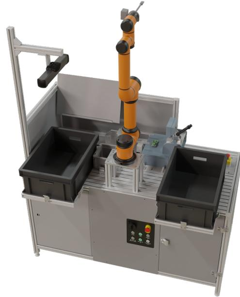
Fig. 2: Render of a PCB testing workplace with the Ensensio 3D camera for bin-picking, 6 DoF Aubo i5 robot, 2 DoF custom-built robot, functional tester, barcode reader, and printer, source, and target boxes.
