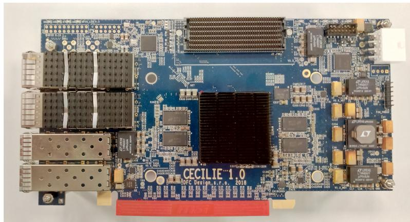
Fig. 3.2: FPGA Network Card [29].
