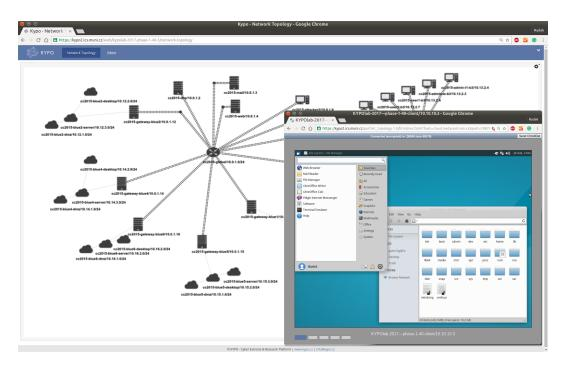
Figure B.3.2: The topology of the exercise network, as seen by participants in the front-end application, and open remote desktop connection to selected host in the separate window.
