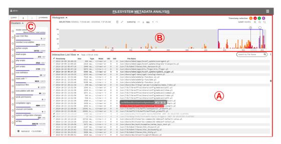
Figure H.0.1: FIMETIS is a tool providing an interactive exploration of file system snapshots. Analysts can quickly investigate cybersecurity incidents via three complementary views: A – *list view* with file system records, B – *histogram* with a timeline, and C – data *clusters*.
