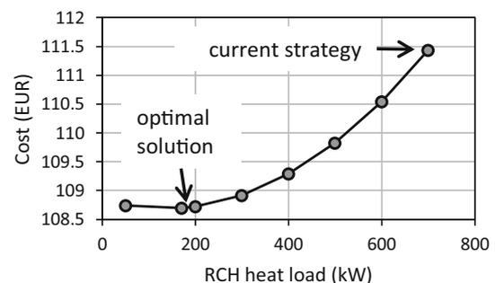
**Fig. 8** Sensitivity of operational costs to RCH load
