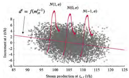
Fig. 5. Drifting probability distribution of increments in steam production.
