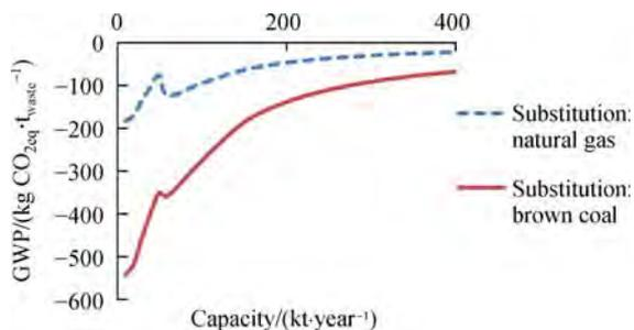
**Fig. 5** Dependence of GWP and capacity
