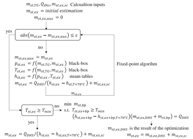
Fig. 7. The algorithm for calculating the extraction steam flow rate.
