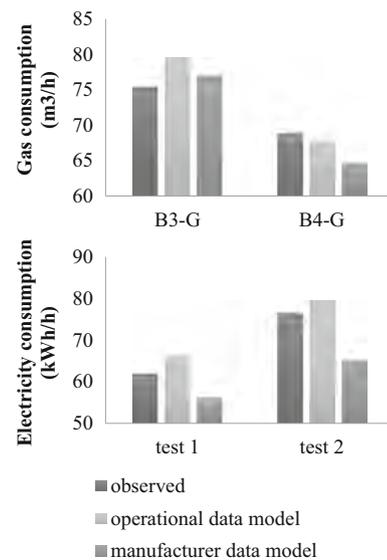
**Fig. 6** Comparison of the developed data-driven models against manually measured values
