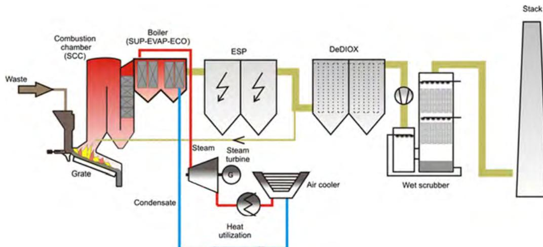
Fig. 2. Block diagram of a WtEP [33].
