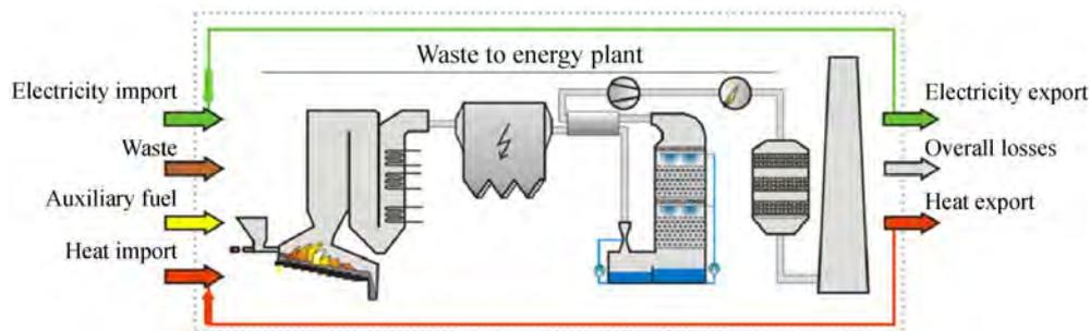
Fig. 2 Simplified diagram of main energy inputs and outputs in WTE plant
