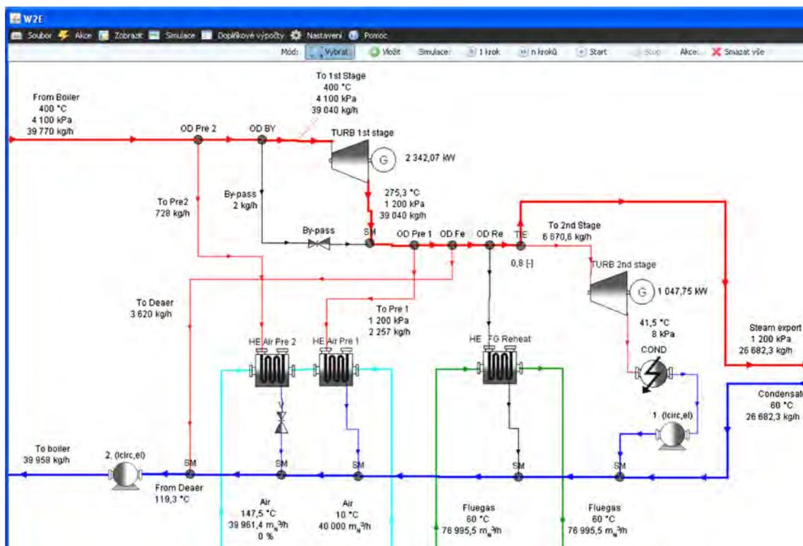
Fig. 3 Simulation model of energy recovery system of WTE plant in in-house software W2E
