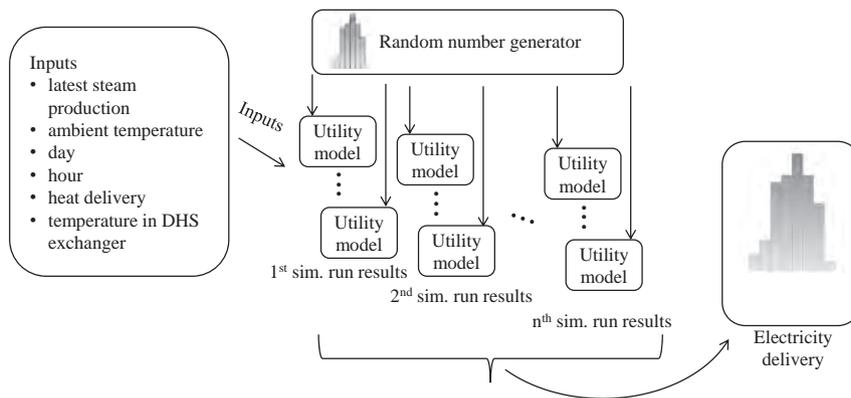
Fig. 9. Scheme of the simulation procedure.
