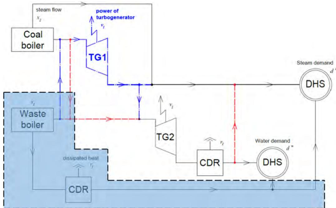
Fig. 11. Scheme of integrated system WtEP and CHPP.
