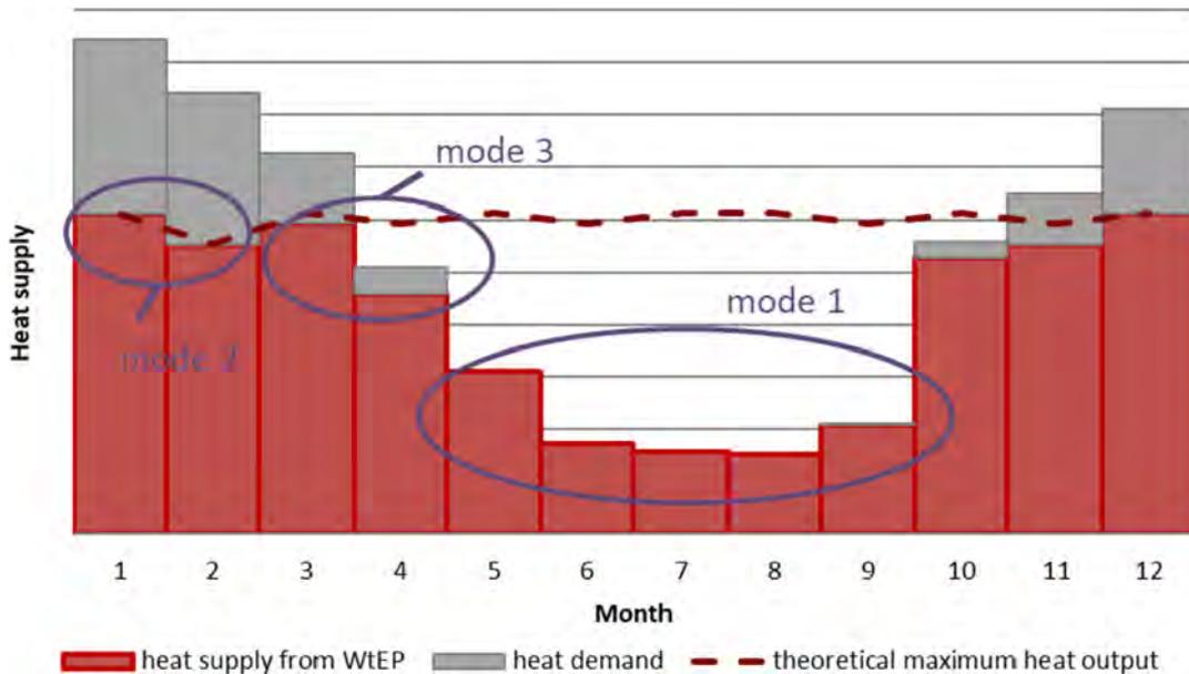
Fig. 3. The three modes with a different relationship between heat demand in the DHS and heat supply from the WtEP.
