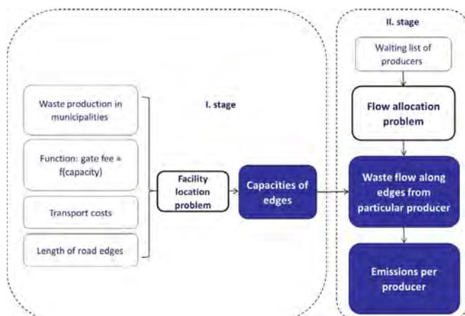
Fig. 4. Modelling of a facility location problem and flow allocation problem.
