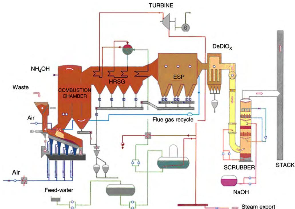
**Fig. 3.** Flowsheet of an up-to-date municipal solid waste incinerator with nominal capacity 100 kt/y.
