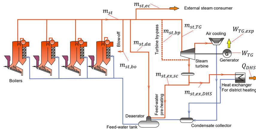
**Fig. 1.** A simplified flow-sheet of the steam–condensate cycle used in WtE technology (red lines represent steam, blue lines represent water, flue gas treatment system excluded). (For interpretation of the references to colour in this figure legend, the reader is referred to the web version of this article.)
