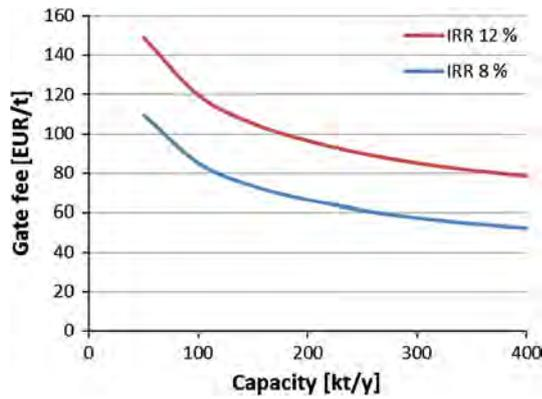
**Fig. 9** An example of capacity-dependent gate fee function generated for one specific project. Uncertainty of future development in key economic parameters is addressed by varying internal rate of return (IRR)
