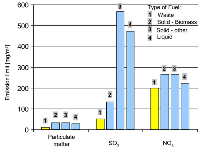
Fig. 2. Comparison of emission limits valid for waste incinerators and other large combustion plants according to fuel used (corrected values for uniform O<sub>2</sub> content 11%) [8,9].
