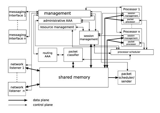
FIGURE 2.4: Active Element architecture
