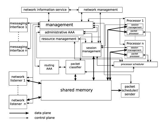
FIGURE 3.1: Architecture of Active Element with Network Management and Network Information Service modules.
