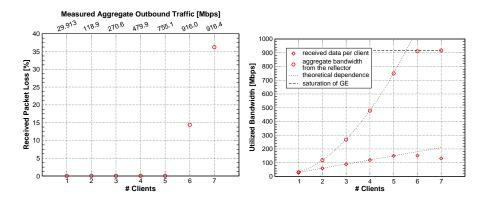
Fig. 2. Reflector prototype performance evaluation for 30 Mbps clients.
