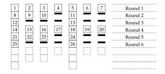
Figure 5: Alternative load balancing packet distribution. Empty round markers are shown as small black filled rectangles.
