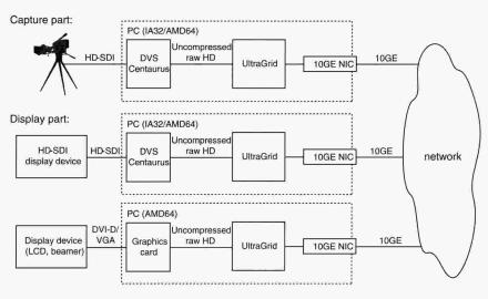
Fig. 1. Site connection scheme for HD transmission.
