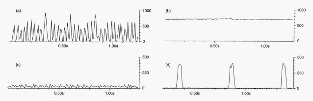
Fig. 4. Bursty traffic produced by the uncompressed HD transport (a) compared to smooth traffic by our measurement probes (b). Bursty traffic produced by the HDV transport with VLC (c) and netcat (d). Vertical axis denotes number of packets per 20 ms interval.
