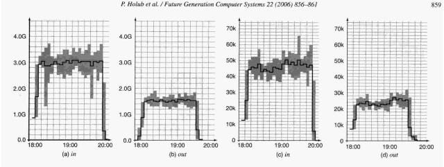
Fig. 3. Network statistics gathered on the Brno uplink. The lines are five minute averages, while the surface is an envelope curve with min/max values within the five minute interval. (a) gives in throughput in Gbps, (b) gives out throughput in Gbps, (c) gives in throughput in packets per second (pps), and (d) gives out throughput in pps.
