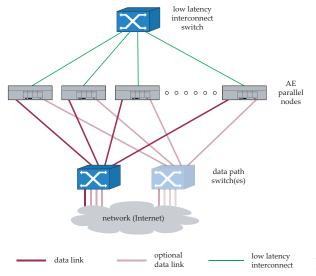
Figure 1: Model infrastructure for implementing the distributed AE.
