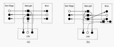
Fig. 2. Connection scheme for (a) the first and (b) the second iGrid experiment. The full lines show uncompressed HD streams; the dotted line shows compressed HDV streams. The empty circles denote sending computers, the full circles stand for display computers, and the full boxes are AEs.
