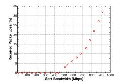
Fig. 3. Raw forwarding performance of the reflector.
