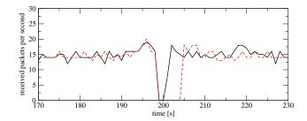
Fig. 1. Recovery time for with backup SPT (solid line) and without it (dashed line) simulated using cnet-based network simulator.
