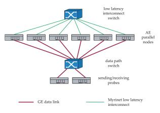
Figure 6: Distributed AE testbed setup.
