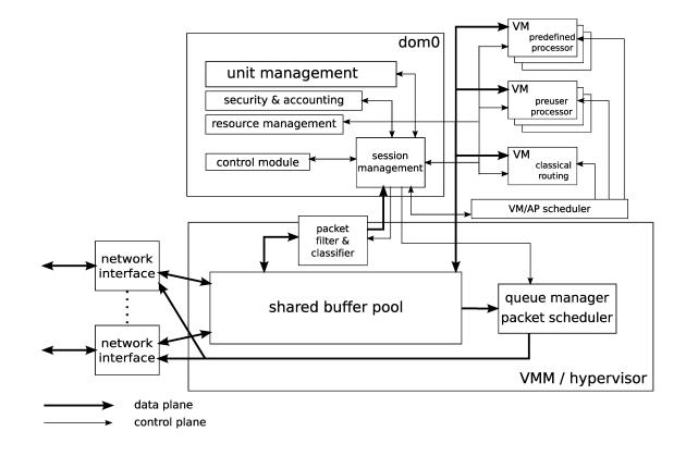
FIGURE 2.3: VM-ready active router architecture
