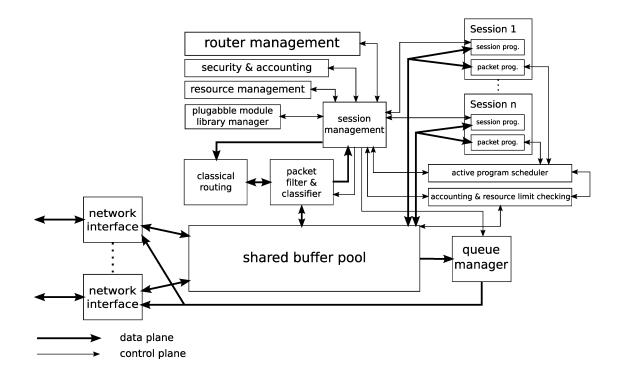
FIGURE 2.2: Model of active router
