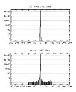
Figure 4. Sample packet reordering distribution with FCT and without synchronization, for 8 parallel units and 3.4 Gbps per data flow.
