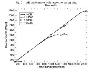
Performance measurement results of the AE are shown in the Figure 2. Exact numbers describing some key points from the graph are summarized in Table I: (a) gives maximum bandwidth of a single stream with packet loss <0.01% with respect to packet size in use, while (b) gives packet loss with
