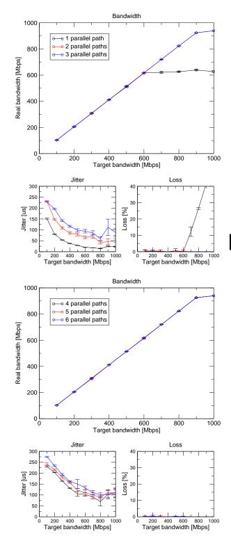
Figure 7: Forwarding performance of distributed AE without explicit synchronization for number of paths 1 through 6.
