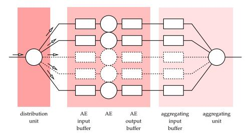
FIGURE 3.2: Model of the distributed AE.
