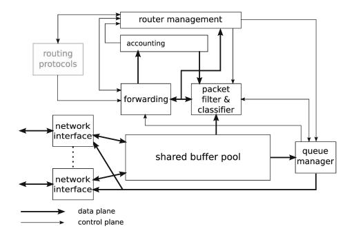
FIGURE 2.1: Model of general router
