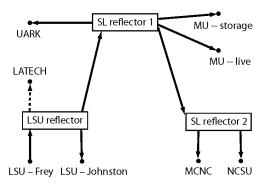
Figure 2: Overlay data distribution network for the 1.5 Gbps uncompressed HD video streams
