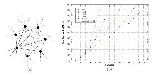
**Fig. 4.** (a) Full mesh reflector tunneling model. (b) Dependence of the number of 30 Mbps clients on the number of reflectors in the mesh.
