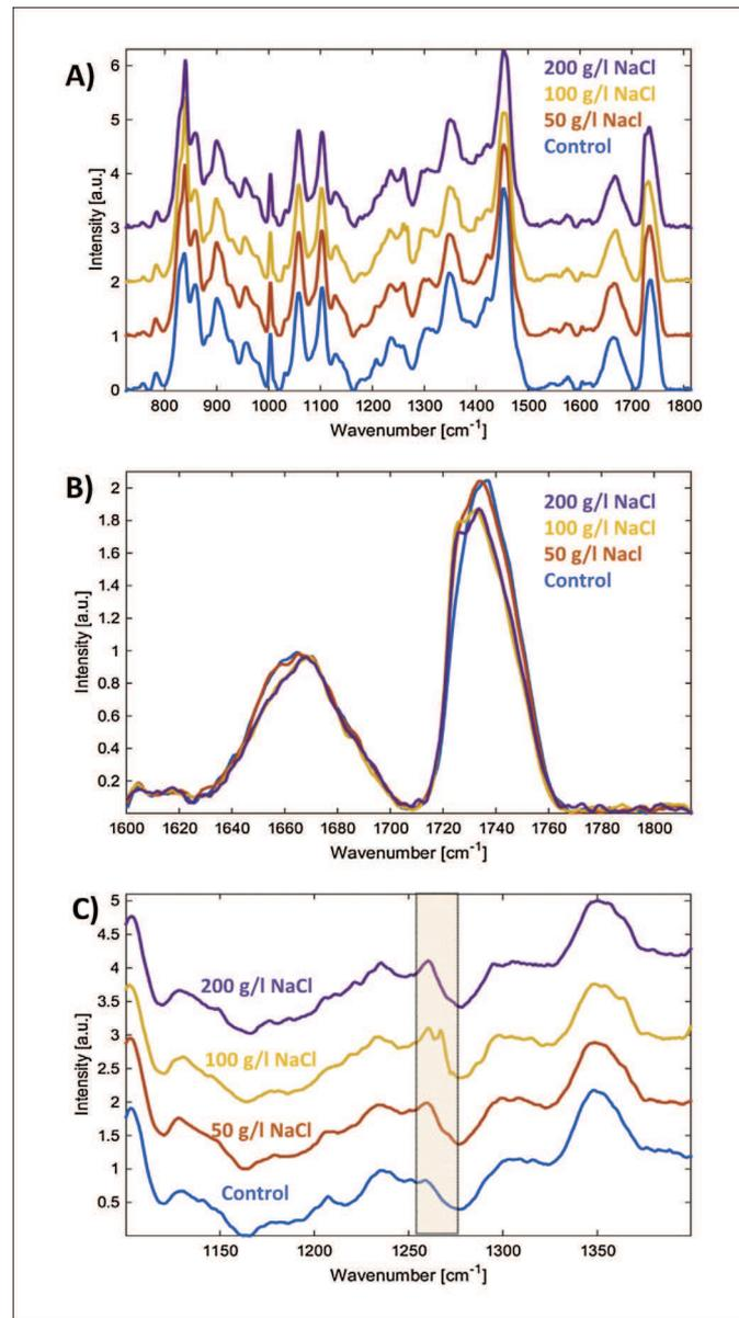
**Fig. 2.** Crystallization of PHB granules of upshocked cells of *C. necator* H16 recorded by Raman spectroscopy. (A) Whole Raman spectrum in the range 800–1800  $\text{cm}^{-1}$ ; (B) detail of crystallization indicating shift of PHB peak at 1736  $\text{cm}^{-1}$  for samples exposed to 100 and 200 g/l NaCl; (C) formation of peak at 1260  $\text{cm}^{-1}$  also indicating partial PHB granule crystallization.
