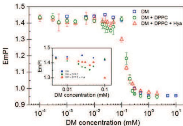
**Fig. 3** Dependences of pyrene EmPI on DM concentration of DM and its mixture with DPPC and DPPC with Hya
