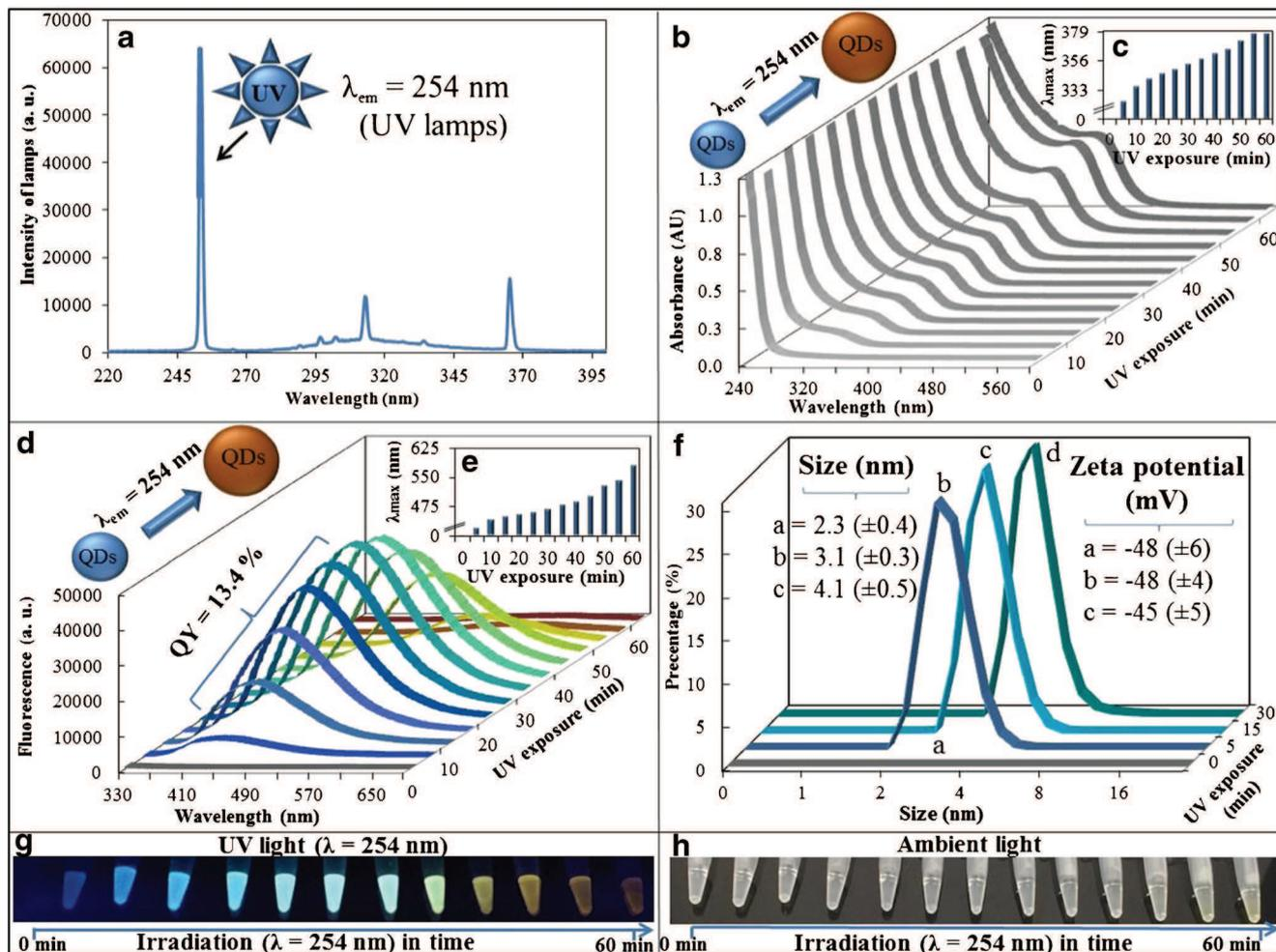
**Fig. 1** Spectral analysis of UV-formed QDs **a** Emission spectrum of UV tubes in the transilluminator, **b** Absorption spectra of CdSe QDs (240–600 nm) obtained after illumination of precursors (0–60 min) by UV light (spectrum shown in 1a), **c** Absorbance maximum shift dependent on illumination time, **d** Fluorescence emission spectra (330–700 nm)
