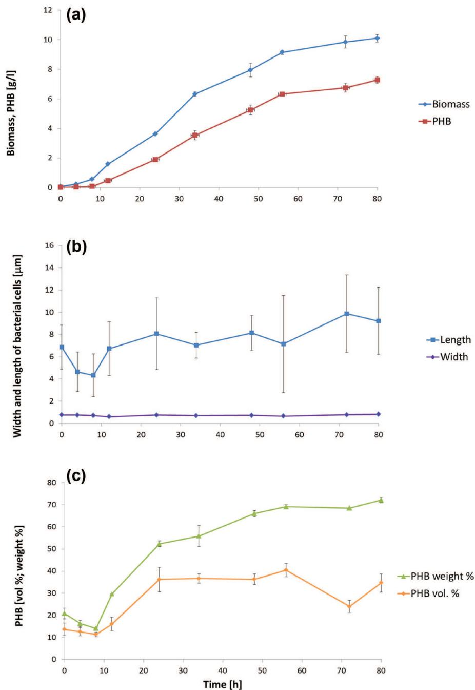
**Figure 3.** Development of following parameters during cultivation of *Cupriavidus necator* H16 in mineral medium with fructose as the sole carbon source (a) biomass and PHA concentration (b) length and width of bacterial cells (c) volume content of PHA granules in cells and weight content of PHA per cell dry weight.
