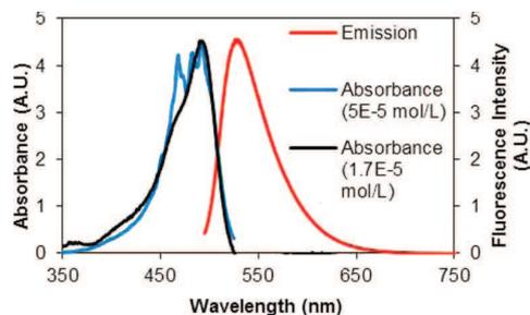
**Figure 2.** Spectral properties of acridine orange in aqueous solution at a concentration of  $5 \times 10^{-5} \text{ mol}\cdot\text{L}^{-1}$  of the dye and the absorption spectrum for the aqueous solution at a concentration of  $1.7 \times 10^{-5} \text{ mol}\cdot\text{L}^{-1}$ .
