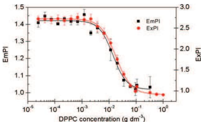
**Fig. 1** Dependence of pyrene EmPI and ExPI on DPPC concentration. The first break in the Boltzmann curve corresponds to the concentration at the beginning of an aggregation (CBA), while the point of inflection corresponds to the  $CAC_{PL}$  of DPPC
