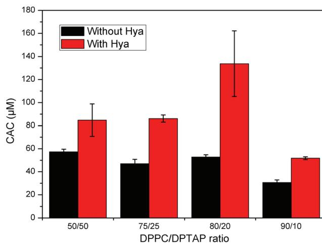
**Fig. 9** Concentration of DPTAP and DPPC at the CAC (determined by pyrene EmPI) of various DPPC and DPTAP mixtures with Hya (15 mg dm<sup>-3</sup>, 458 kDa)
