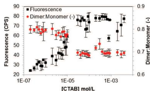
**Figure 7.** Dependencies of the fluorescence intensity and dimer:monomer ratio as a function of CTAB concentration in the AO–hyaluronan–CTAB system (concentrations of AO and hyaluronan correspond to the equivalence point  $(P/D)_e = 3$ ).
