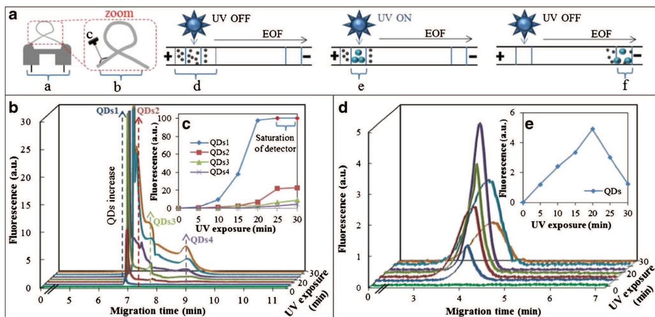
**Fig. 3** a Scheme of modified capillary pathway and special window position, a) conventional capillary cartridge with the capillary inside the cooling tube, b) capillary directed out of the cooling tube, c) UV LED ( $\lambda_{em} = 250$  nm) connected to the optical fiber focusing the light into the capillary, d) zone of QD precursors injected into the capillary UV LED off, e) formation of QDs using UV LED on, f) CE separation of formed QDs and LED-LIF detection by 380 nm LED
