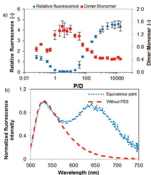
**Figure 8.** (a) Ratio of relative fluorescence and absorbance (D:M) of acridine orange monomer and dimer in the PSS-AO system. Fluorescence is relative to the sample in which PSS is not present. (b) Emission spectrum of acridine orange from a sample without PSS and with PSS (at the equivalence point determined in this section,  $P/D = 4$ ).
