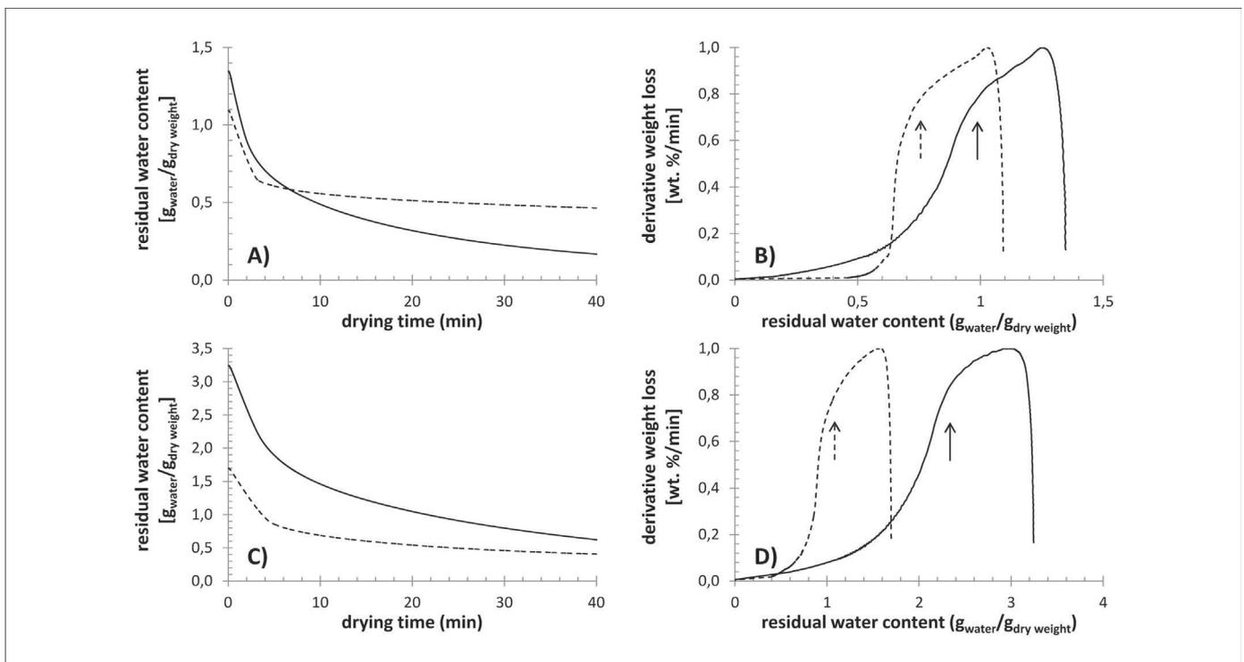
**Fig. 7.** The effect of osmotic challenge on drying curves determined by isothermal TGA experiments at  $60\text{ }^{\circ}\text{C}$  on *C. necator* H16 (A, B) and *C. necator* PHB-4 (C, D). Solid lines represent unchallenged bacterial samples, dashed lines represent samples exposed to  $200\text{ g/L}$  NaCl. The heights of the derivative weight loss curves (B, D) were normalized for clarity. Arrows indicate respective critical water contents.
