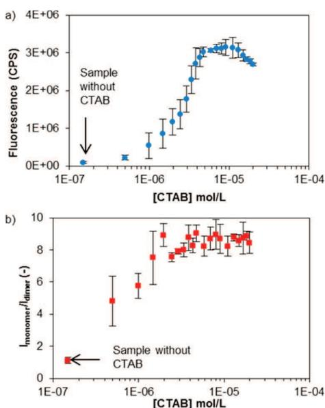
**Figure 9.** (a) Plot of the acridine orange fluorescence intensity as a function of increasing CTAB concentration. (b) Plot of the AO monomer/dimer fluorescence intensity ratio as a function of surfactant concentration. The concentrations of AO and PSS were held constant in all samples.
