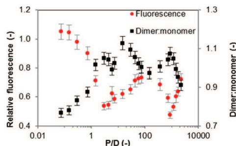
**Figure 4.** Comparison of dependencies of the relative fluorescence intensity and dimer:monomer ratio on the  $P/D$ . The concentration of hyaluronan covers the range from  $0.5 \text{ mg L}^{-1}$  to  $15 \text{ g L}^{-1}$ . Fluorescence is relative to the sample in which hyaluronan is not present.
