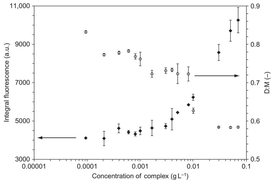
**Figure 11** Dependency of the fluorescence intensity of acridine orange (as total integral; ◆) and D:M (○) ratio on concentration of DPPC–C<sub>12</sub>maltoside complex.
