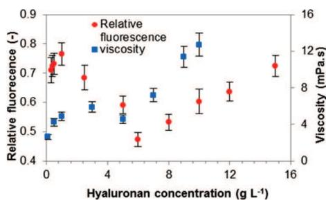
**Figure 6.** Dependencies of the fluorescence intensity and viscosity obtained from microrheology experiments on the hyaluronan concentration. Fluorescence is relative to the sample in which hyaluronan is not present.
