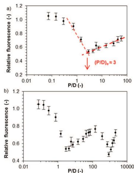
**Figure 3.** Dependency of the relative fluorescence intensity on the P/D of the system with a constant concentration of acridine orange of  $1.7 \times 10^{-5} \text{ mol}\cdot\text{L}^{-1}$ . Fluorescence is relative to the sample in which hyaluronan is not present. The concentration of hyaluronan in (a) covers the range from 0.5 to  $400 \text{ mg}\cdot\text{L}^{-1}$ . In (b), we expanded the concentration range up to  $15 \text{ g}\cdot\text{L}^{-1}$ .
