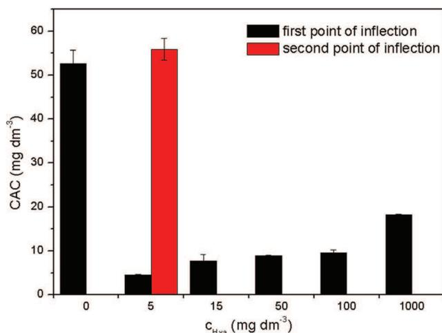
**Fig. 6** CAC of DPTAP and Hya mixtures with different Hya concentrations determined by pyrene EmPI. In the case of a Hya concentration of  $5 \text{ mg dm}^{-3}$ , a double Boltzmann curve was used to fit the dependence of pyrene EmPI on DPTAP concentration, and two points of inflection were obtained
