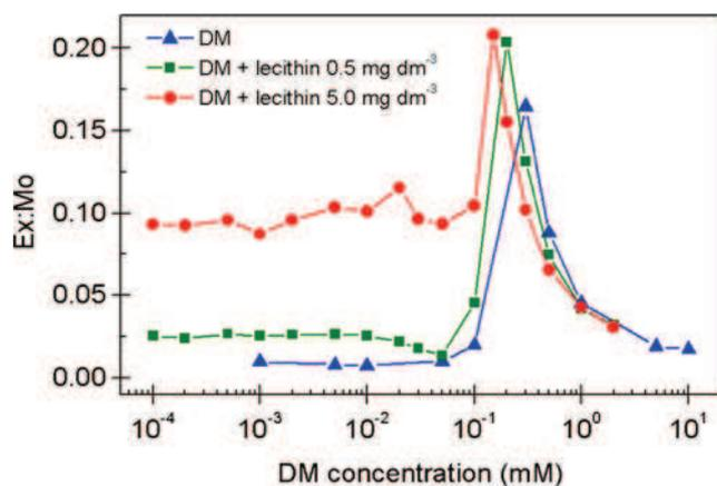
**Fig. 6** Dependences of pyrene Ex/Mo on the DM concentration of DM and on the DM concentration of DM mixtures with lecithin at a concentration  $0.5 \text{ g dm}^{-3}$  and with lecithin at a concentration of  $5.0 \text{ g dm}^{-3}$
