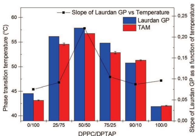
**Fig. 3** Phase transition temperature in DPPC/DPTAP vesicles obtained using laurdan generalized polarization and microcalorimetry and the slope (absolute value) of the dependence of laurdan GP on temperature
