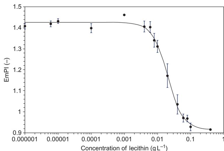
**Figure 5** Dependency of the emission polarity index (EmPI) on concentration of lecithin. Data were fitted by Boltzman sigmoidal curve and fitted parameters were used to characterize aggregation process of lecithin, see [Table 2](#).
