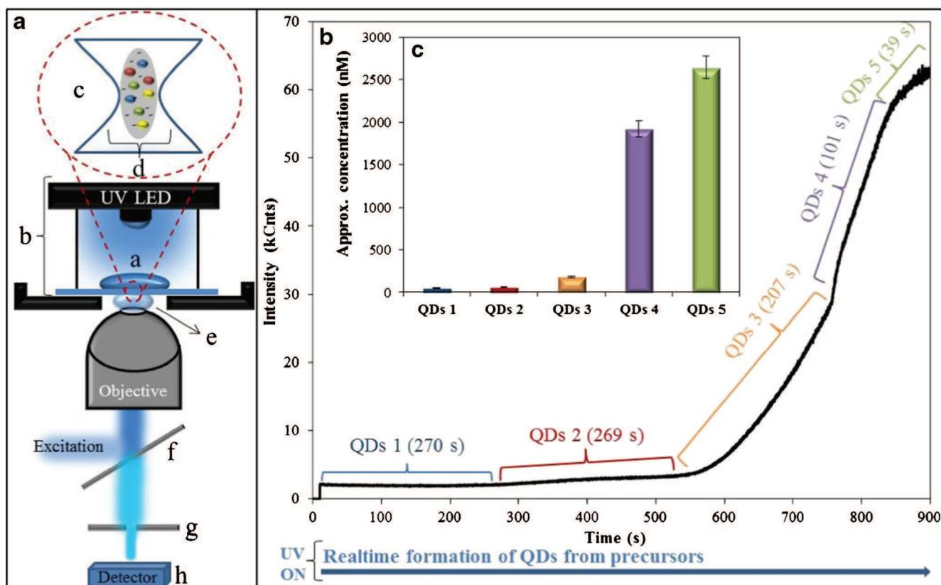
**Fig. 2** a Schematic representation of the UV LED modified FCS a) 15  $\mu$ L drop of precursors (Cd:Se) on quartz glass, b) UV LED ( $\lambda_{em} = 250$  nm), c) idealized confocal volume, d) schematic representation of the QDs formation in a confocal volume, e) lens with water immersion, f, g) laser ( $\lambda_{em} = 367$  nm, 1 MHz repetition), optical
