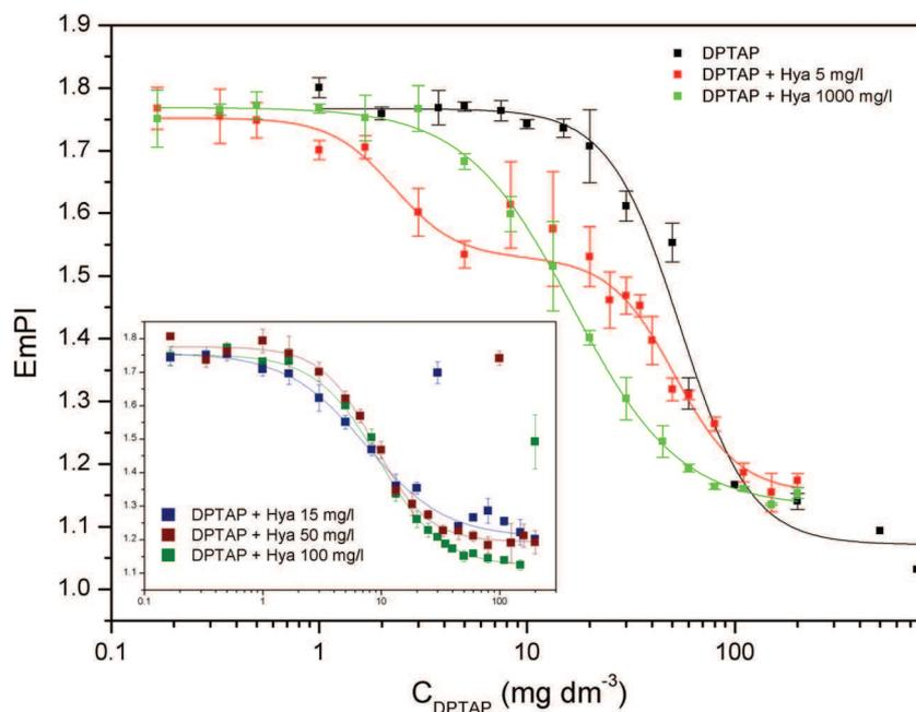
dependence corresponding to DPTAP has a sigmoid character, with high EmPI values at low DPTAP concentrations indicating fluorescence from a polar (water) environment. At high DPTAP concentrations, EmPI values are low, because fluorescence occurs from the hydrophobic region.
