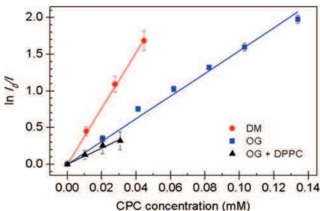
**Fig. 5** Dependences of  $\ln I_0/I$  on CPC concentration for determination of the aggregation numbers of DM, OG, and the mixture of OG and DPPC
