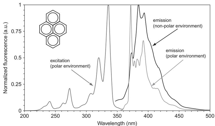
**Figure 2** Fluorescence properties of pyrene in environments of different polarity.
