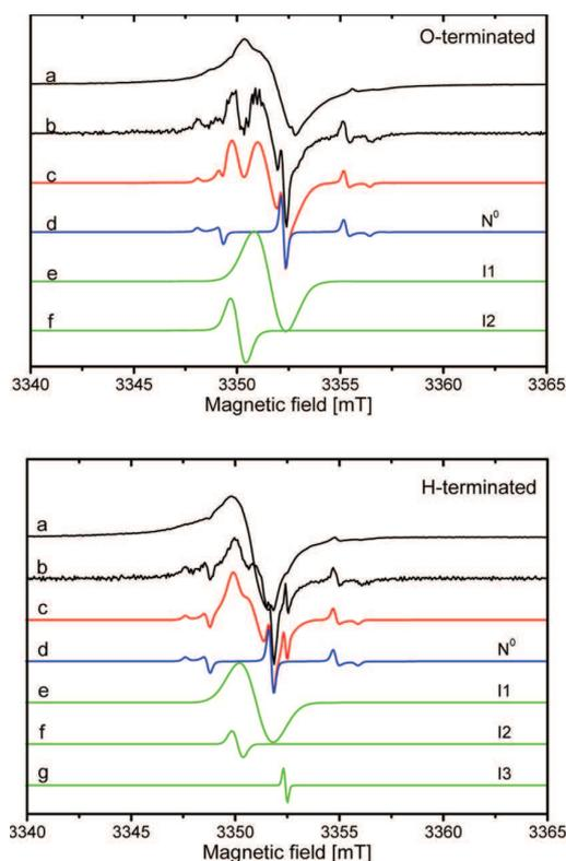
**Figure 3.** Experiment/simulation of two differently terminated ND samples: (top) O-terminated and (bottom) H-terminated: CW EPR (a) and the first derivative ESE-detected EPR (b) spectra, sum of simulated EPR spectra components (c), simulated  $N^0$  center (d), and I1–I3 simulated components (Voigtian line shape) of EPR spectra (e–g); W-band,  $T = 50$  K.
