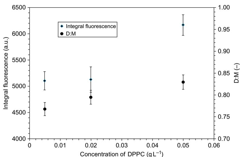
**Figure 8** Dependency of the fluorescence intensity of acridine orange (as total integral) and D:M ratio on concentration of DPPC in the presence of hyaluronan (MW 73,000 g mol<sup>-1</sup>; 15 mg L<sup>-1</sup>).
