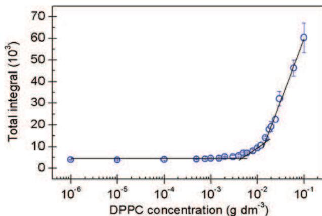
**Fig. 2** Dependence of total integral of Nile Red emission spectra on DPPC concentration, fitted by three straight lines. The first point of intersection corresponds to CBA, while the second corresponds to  $CAC_{PL}$  of DPPC
