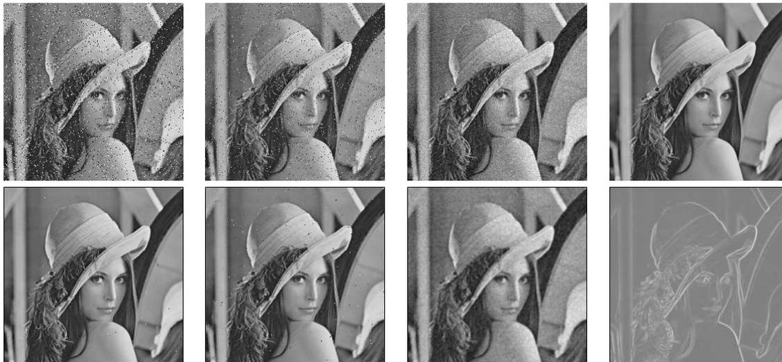
**Table 5.8.** Corrupted and filtered images: Salt and pepper noise, random shot noise, Gaussian noise, edge detector
