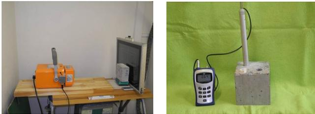
Fig. 2. X-ray machine EcoRay HF 1040 with digital recording to PC equipment (left photo). PeMaSo-01 depth probe for magnetic measurements (right photo).
