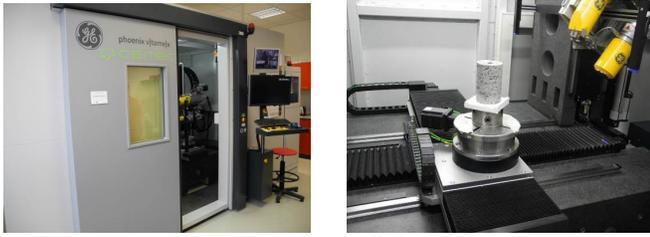
Fig. 6. Tomograph GE phoenix.v|tome|xL 240 (left photo) and a cylindrical specimen fixed in its manipulator (right photo).
