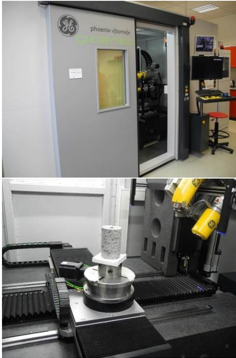
Figure 6: Tomograph GE phoenix,v|tome|x L 240 (left photo) and a cylindrical specimen fixed in its manipulator (right photo).
