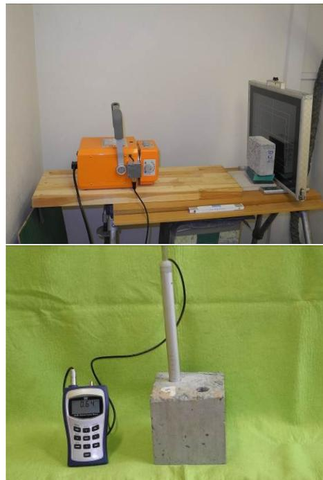
Figure 2: X-ray machine EcoRay HF 1040 with digital recording to PC equipment (left photo). PeMaSo-01 depth probe for magnetic measurements (right photo).
