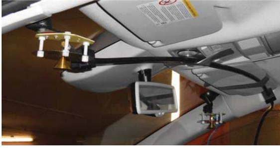
(a) 3-11 GHz monoconical antenna mounted on front windshield next to the rear-view mirror.
