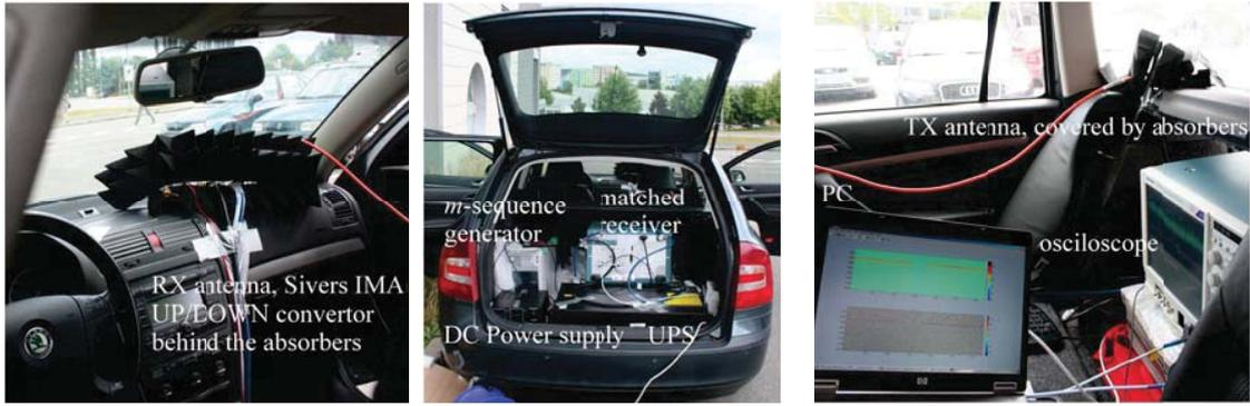
(a) The dashboard of the measurement vehicle. Behind the absorbers is the RX with both the up/down Siviers IMA converters and the LNA.
