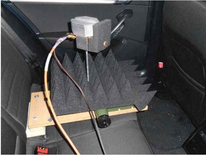
(c) X-Y table for precise movement of the open-ended waveguide antenna within the measurement grid. The metallic X-Y table, the antenna with power amplifier and heat sink are covered with absorbers in order to reduce the unwanted reflections and thus the influence of the measurement. The grid position corresponds to  $\kappa = 1$ .
