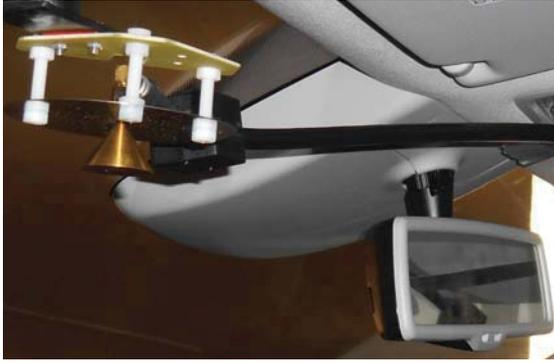
(a) 3-11 GHz monoconical antenna mounted on the front windshield next to the rear-view mirror.
