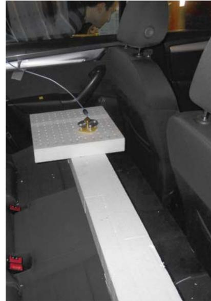
(d) Polystyrene  $10 \times 10$  antenna holder and 3-11 GHz monoconical antenna. The grid position corresponds to  $\kappa = 1$ .
