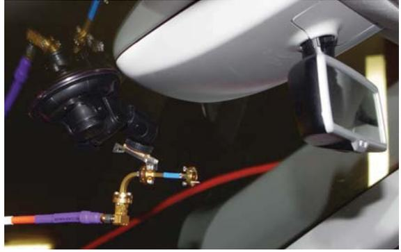
(b) 55-65 GHz open-ended waveguide antenna fastened using a suction cap.
