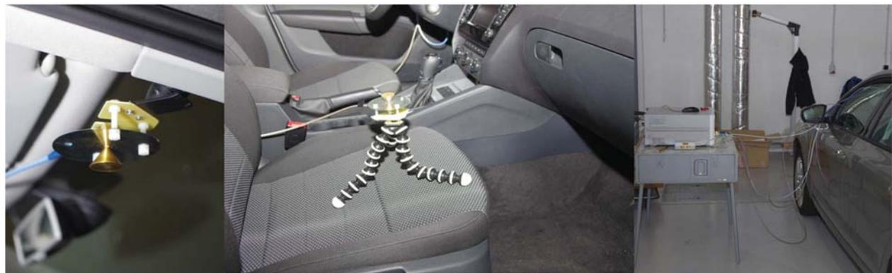
**Figure 2** Images of the conical monopole antenna, measurement position, and four-port VNA. [left] Detail of the conical monopole antenna mounted on the front windshield. [middle] One measurement position inside the vehicle. [right] Four-port VNA connected with antennas inside the measured vehicle.
