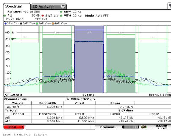
Figure 8.4: The power spectrum density where green trace represents FBMC signal without DPD, black signal is FBMC signal with DPD and blue curve is OFDM signal without DPD. The signals were obtained at the output of PA denoted as Mini Circuits with input power  $P_{IN} = -14dBm$ .
