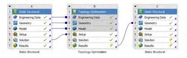
Figure 5.4: Classical topology optimization work-flow in Ansys Workbench 19.1. Figure by author.
