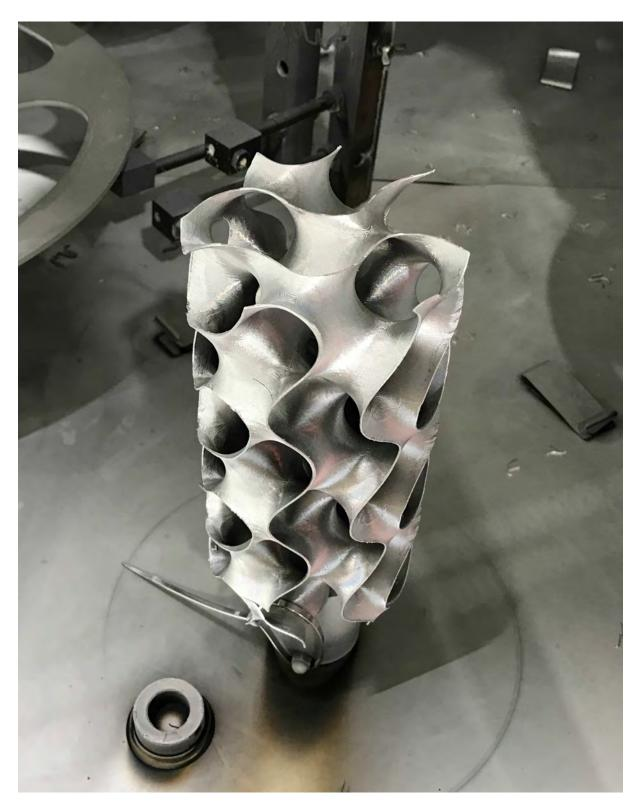
Figure 10.6: Vacuum coating of the gyroid surface without the cylindrical confinement jacket. Photographed by the author in 2018.
