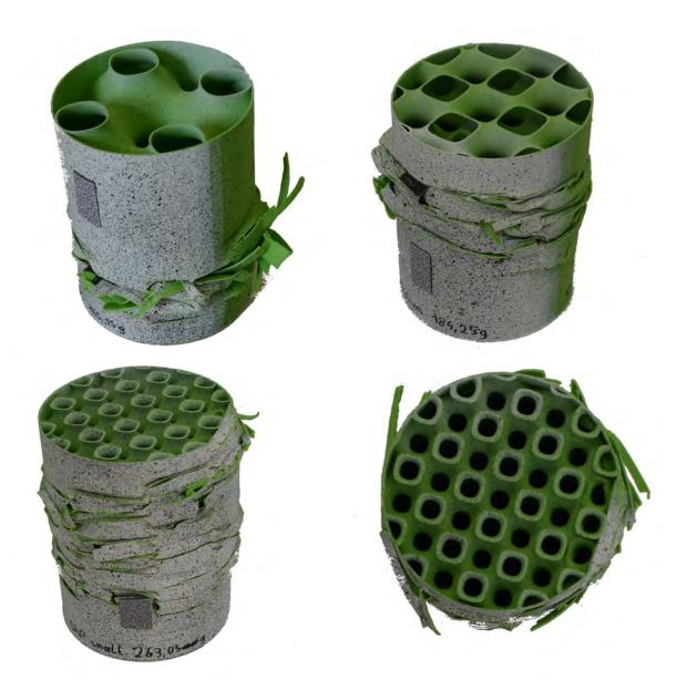
Figure 9.11: Sample realizations of cylinder compression tests with 3 scales of 3D Schwarz P infill. Photographed by the author in 2018.
