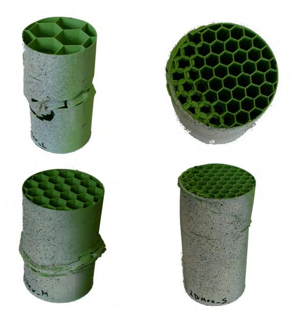
Figure 9.8: Sample realizations of cylinder compression tests with 3 scales of reference 2D honeycomb infill. Photographed by the author in 2018.
