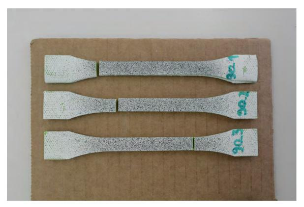
Figure 9.13: Three realizations of ISO dogbone specimens sliced according to DB 90 after the tensile test. Photographed by the author in 2018.
