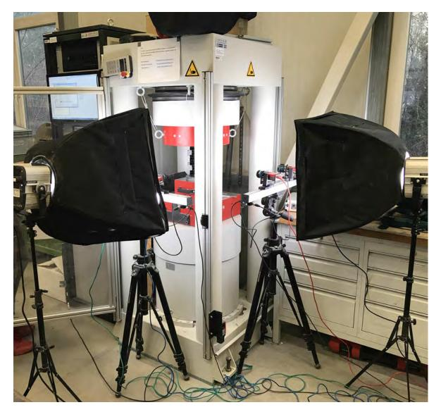
Figure 9.6: Hydraulic compression testing machine controlled by a prescribed displacement rate in combination with a 3D digital image correlation (DIC) system enabling to record full strain fields and objectively interpret the load-displacement diagrams and stiffness. Photographed by the author in 2018.
