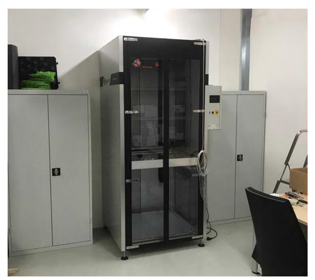
Figure 9.1: Industrial grade large scale FDM 3D printer Builder 2000. Photographed by the author in 2018.
