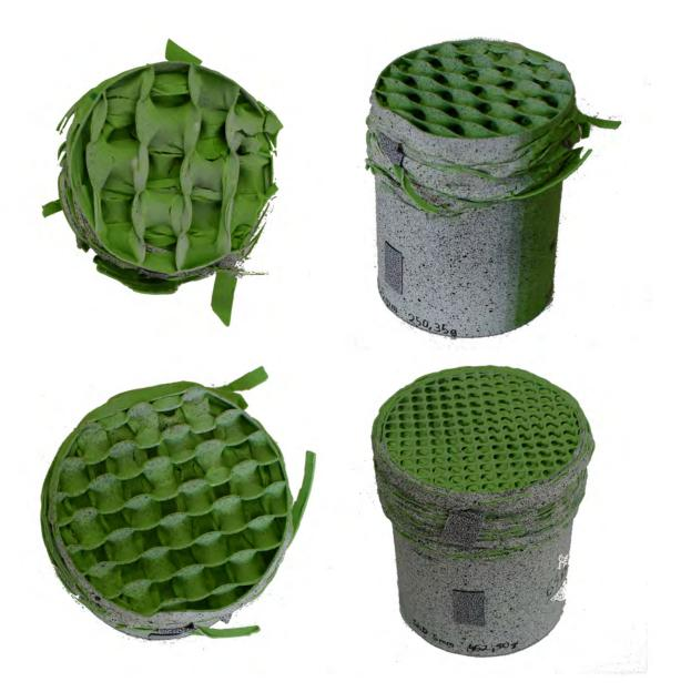
Figure 9.10: Sample realizations of cylinder compression tests with 3 scales of 3D Schwarz D infill. Photographed by the author in 2018.
