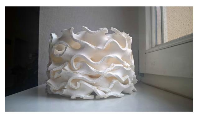
Figure 7.7: Gyroid sample printed from PLA after the compression test. Figure by author.
