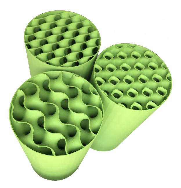
Figure 8.2: Example of 3D printed 3D infill patterns (Schwarz P, Schwarz D and Gyroid at medium scale) generated inside a cylinder. Photographed by author in 2018.
