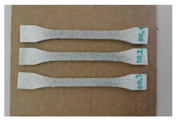
Figure 9.12: Three realizations of ISO dogbone specimens sliced according to DB 00 after the tensile test. Photographed by the author in 2018.
