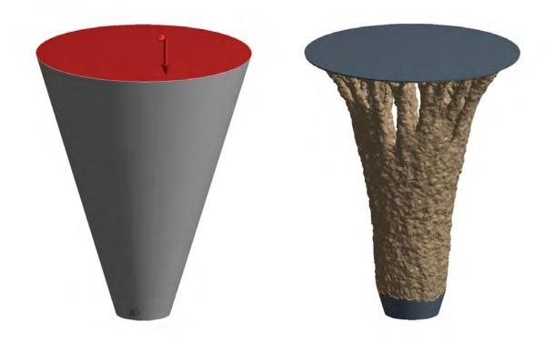
Figure 5.5: Classical topology optimization principle: initially defined solid body with boundary conditions (left) and the retained 15% mass after iterative removal of least stressed elements. Figure by author.
