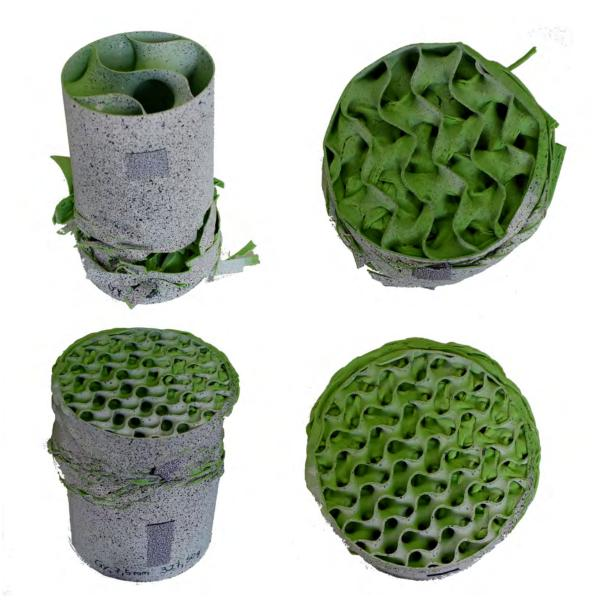
Figure 9.9: Sample realizations of cylinder compression tests with 3 scales of 3D gyroid infill. Photographed by the author in 2018.
