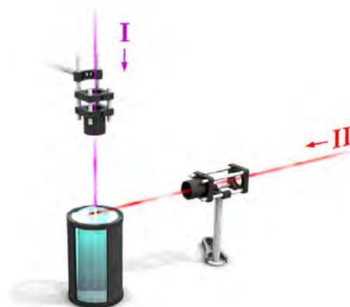
Fig. 2. Schematic diagram of experimental setup for bulk liquid LIBS experiments involving the two lasers. Ablation laser I (from the top) at 266 nm and re-heating laser pulse II (from the side) at 1064 nm are shown.
