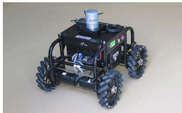
▲ **ATEROS** – The Autonomously Telepresence Robotic System was one of the winners of the **Golden Ampere 2017** competition. The System was created at BUT by the working group of Luděk Žalud. ATEROS is a multi-robotic system for autonomous exploration of places that are inaccessible or dangerous to people. The system can automatically create 3D maps of the area and can also search for people.
