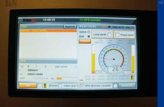
A new intelligent lubrication system of the flanges of rail vehicles, which eliminates unpleasant noise, and automatically calculates the lubricant doses using GPS data, was developed by scientists from the Institute of Design at the Faculty of Mechanical Engineering.
